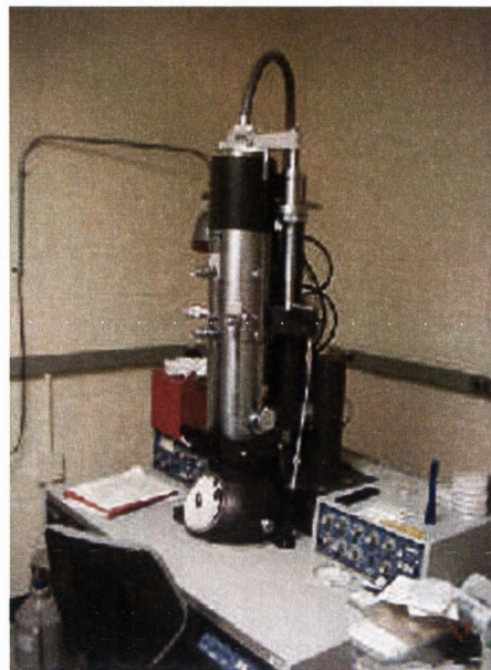
Figure 1.6: LHS: HRTEM image of circular CdS nanocrystals in the 5.5nm size range. Note: It is possible to see the crystal lattices of individual particles using this technique. RHS: Picture of a standard transmission electron microscope (TEM) www.micro.cornell.edu/IMAGES/TEM.sized.jpg .
