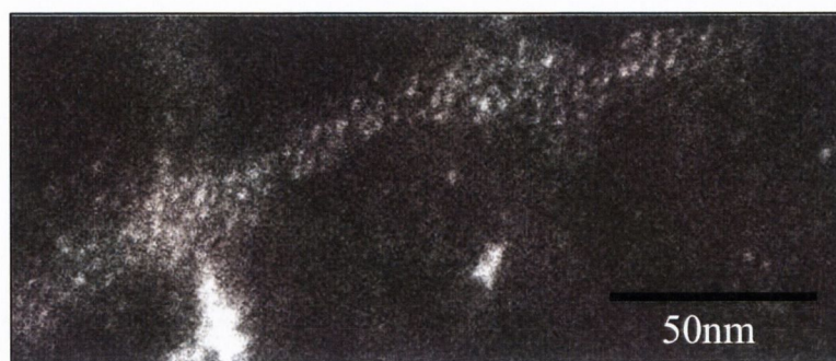
Figure 4.12: ADF image for R-Penicillamine- stabilised CdSe. 5nm particles aggregate into 30-70nm long needle-like assemblies.
