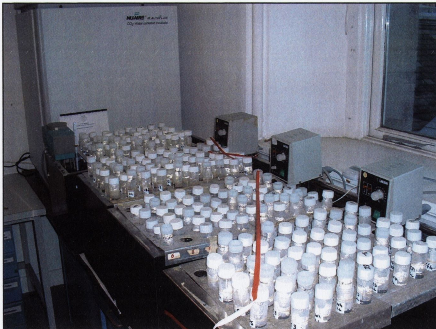
Plate 3.2.2: Baermann tubes set up in water baths in laboratory
