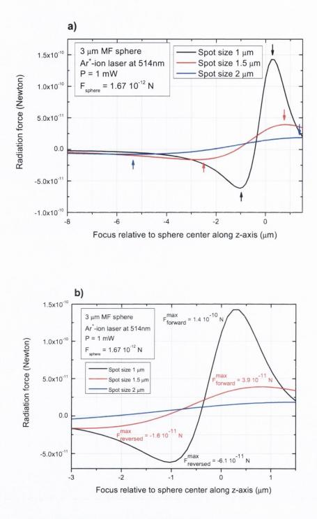
**Figure 2.** Calculated radiation force as a function of the focus position along the z-axis. The sphere centre corresponds to z = 0. The calculation is carried out for a 3  $\mu$ m sphere for 3 different spot sizes. Arrows in a) indicate the radiation force maxima, while the peak labels in b) give the magnitude of the maximum radiation force at the peak points.
