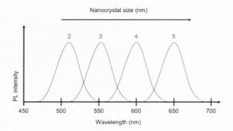
*Figure 2.* Size-dependent luminescence of colloidal thioglycolic acid capped CdTe nanocrystals.
