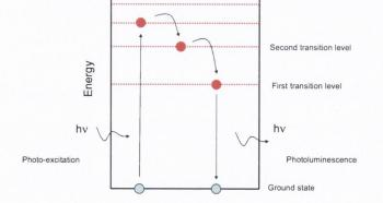
Figure 2. Schematic of photo-excitation and photoluminescence in a quantum dot.
