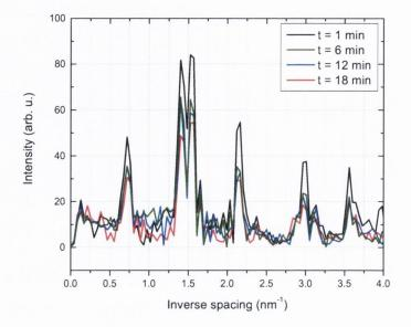
*Figure 14.* Fourier spectrum of the first half of the photoluminescence spectrum at 10% laser intensity for four measurements taken during excitation.
