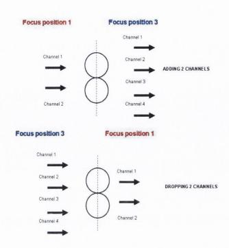
*Figure 8.* Principle application of the optical switch. The spectra are shown in Fig. 7. According to the focus position, the bi-sphere systems works as a add/drop filter.
