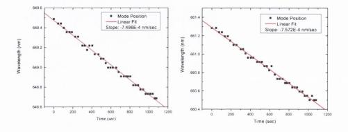
*Figure 17.* Wavelengths of resonance modes plotted versus the excitation time at continuous laser excitation at 0.3 mW laser output power.
