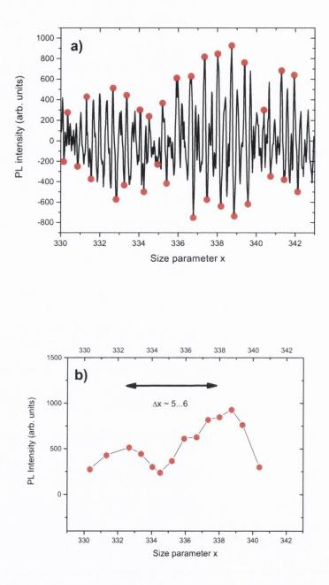
**Figure 5.** Interference structure of the resonances in the PL spectrum. a) Spectrum with peak maxima and minima (red dots), determined with a programme. b) Plot of peak maxima without PL spectrum.
