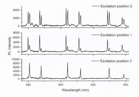
*Figure 9. PL spectra of a bi-sphere system, excited at 3 different positions according to Fig. 6. The diameter difference between the two spheres is 10 nm.*
