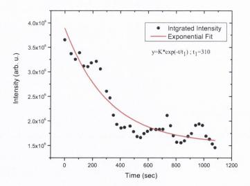
Figure 11. Decay of integrated intensity over time at 0.3 mW HeNe laser output power.
