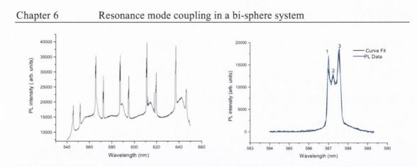
*Fig. 2. left: PL* measurement of a WGM spectrum of a single sphere on a polystyrene substrate. *right:* Lorentzian curve fit of a single peak from the spectrum.
