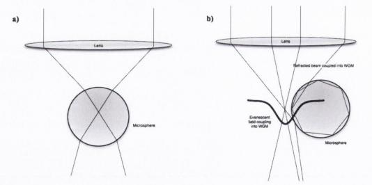
*Figure 8. a)* On-axis focus of laser beam, light is refracted through the microsphere. b) Off-axis focus of laser beam. Evanescent coupling and coupling through refraction.
