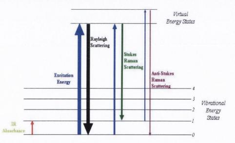
*Figure 1.* Schematic illustration of Rayleigh scattering, Stokes and anti-Stokes Raman scattering.
