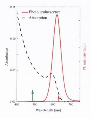
*Figure 3.* Arrows indicate off-resonance (red arrow, HeNe laser at 632.8 nm) excitation and resonance (green arrow, Ar+-ion laser at 488 nm) excitation.
