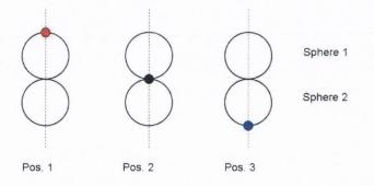
*Figure 6.* Excitation spots for experimental channel switching in a bi-sphere system: top edge of sphere 1 (red spot), in between sphere 1 and sphere 2 (black spot) and bottom edge of sphere 2 (blue spot).
