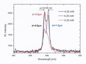
*Figure 25.* Two-channel optical switch realised by a variation of the focus position and consequently, the radiation pressure.
