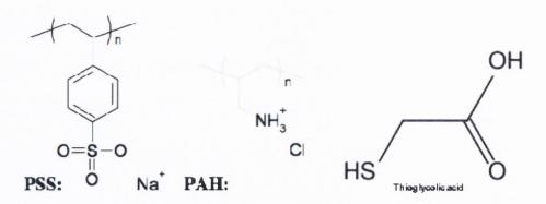
**Figure 1.** Chemical composition of the polyelectrolytes used for the multilayers (PSS and PAH) and chemical formula for thioglycolic acid (capping agent of the colloidal CdTe nanocrystals).
