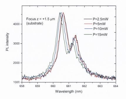
*Figure 12. TE mode of PL measurements at constant focus with variation in laser output power.*
