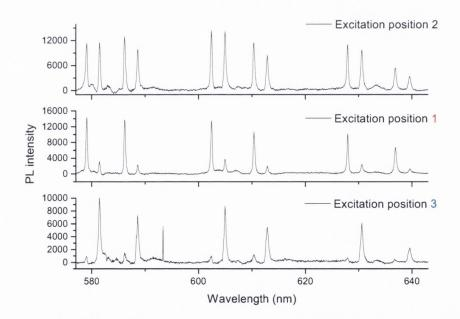
*Figure 10. PL spectra of a bi-sphere system, excited at 3 different positions according to Fig. 6. The diameter difference between the two spheres is 24 nm.*
