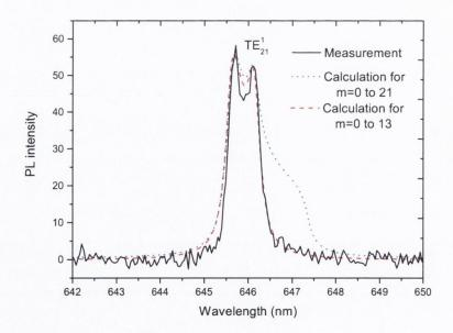
Figure 15. Measured and modelled TE resonance mode.
