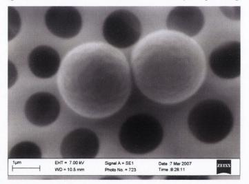
**Figure 1.** SEM picture of a bi-sphere placed on the polystyrene pore substrate. The spheres are located on the pores to reduce the contact with substrate and consequently the leakage of light which quenches the Q-factor.
