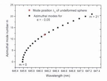
Figure 17. Calculated azimuthal mode positions for the resonance peak in Fig. 15.
