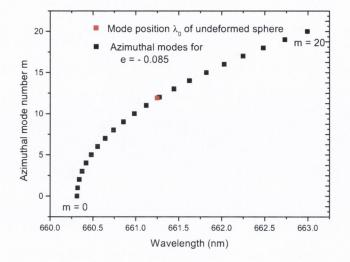
Figure 16. Calculated azimuthal mode positions for the resonance peak in Fig. 14.
