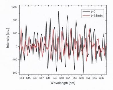
**Figure 16.** PL spectra of 70 µm spheres at the beginning of the continuous excitation (black line) and after 18 minutes of excitation (red line) at 3 mW laser output power.
