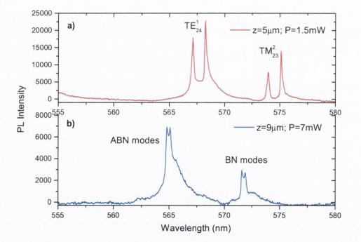
*Figure 4.* a) Separated TE and TM peaks of both spheres due to size difference under weak coupling conditions. b) ANB and BN modes under strong coherent coupling. The z-value state the relative focus position above the substrate.
