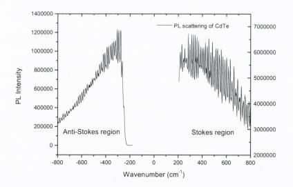
*Figure 6. PL spectrum of CdTe nanocrystals coupled to a spherical microcavity with 70* µm diameter. Excitation with a HeNe laser at 10 mW.
