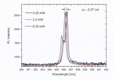
Figure 24. Resonance mode tuning by the variation of the laser intensity.
