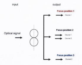
*Figure 11.* Schematic configuration of an optical switch based on a weakly coupled bi-sphere (Fig. 9 and 10). Depending on the focus position according to Fig. 6, the signal is coupled into either both optical channels or one single channel.
