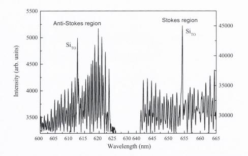
*Figure 4.* Photoluminescence spectrum excited off-resonance with a HeNe laser at P = 3 mW output power.
