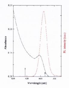
*Figure 1.* Absorption and photoluminescence spectrum of CdTe nanocrystals in aqueous solution.
