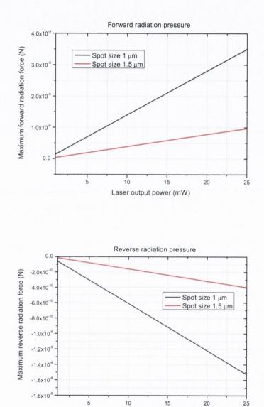
Figure 3. Maximum forward and reverse radation pressure for 2 different spot sizes.
