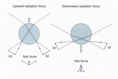
*Figure 1.* Reverse and forward radiation pressure as a result of the gradient force. The momentum change  $\Delta p$  of the refracted beam is transferred to the particle.
