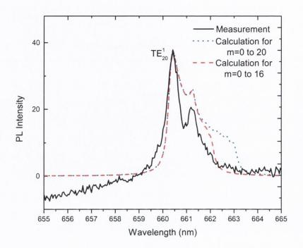
Figure 14. Measured and modelled TE resonance mode.
