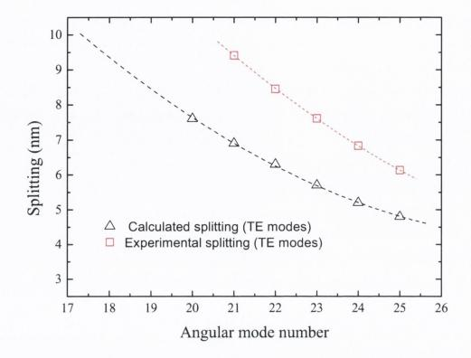
*Figure 5.* Theoretical and experimental spacing between BN and ABN modes as a function of the angular mode number.
