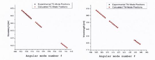
*Figure 10.* Identified first order TE and TM resonances in the PL spectrum in regards of the angular mode number  $\ell$ .
