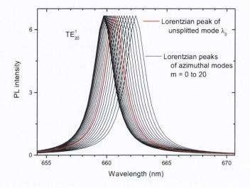
**Figure 19.** Plot of all individual azimuthal modes which result in the modelled peak of Fig. 14. the red peak corresponds to the original unsplitted mode  $\lambda_0$ .
