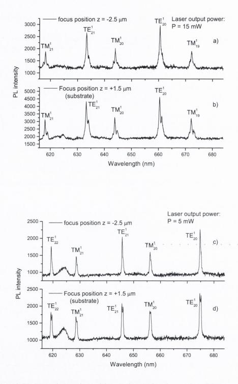
**Figure 9.** PL spectra of microspheres while trapped in a cw laser beam under radiation pressure. (a) and (b) Same microsphere sample (4 bi-layers), excitation power P = 15 mW taken at different focus positions. (c) and (d) Another microsphere sample (5 bi-layers) modified with a salt solution and taken at considerably lower excitation power P = 5 mW, also at different focus positions.
