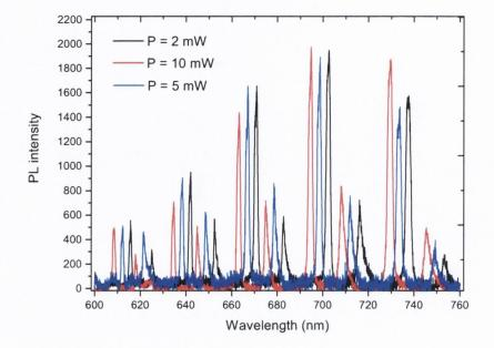
*Figure 23.* Blue-shift of resonances in a 3 micron sphere placed on a gold mirror substrate.
