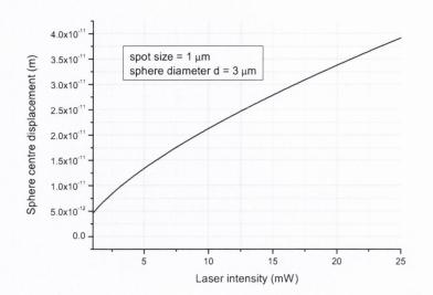
**Figure 4.** Intensity-dependent sphere deformation in polar direction for a 3  $\mu m$  MF sphere.
