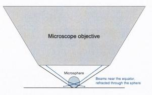
**Figure 18.** Microsphere in a tightly focused laser beam. The focused light near the equatorial region is more likely to be refracted through the sphere, than coupled into the high m azimuthal modes.
