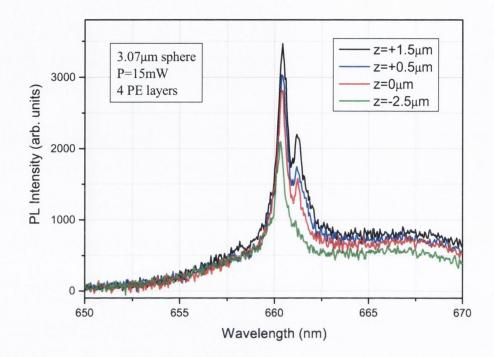
Figure 10. TE mode of the PL spectrum in Fig. 8 b) for 4 different focus positions.
