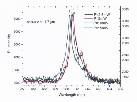
*Figure 13. TE mode of PL measurements at constant focus with variation in laser output power.*
