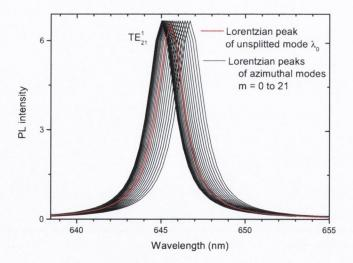
**Figure 20.** Plot of all individual azimuthal modes which result in the modelled peak of Fig. 15. the red peak corresponds to the original unsplitted mode  $\lambda_0$ .
