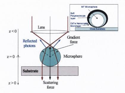
Figure 8. Experimental scheme of the radiation pressure experiment.
