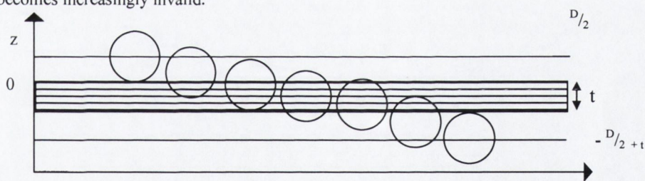
Figure 2. 6. Figure schematically illustrating the manner in which the projected area in TEM image is sensitive to the section thickness of the microtomed coupe.
