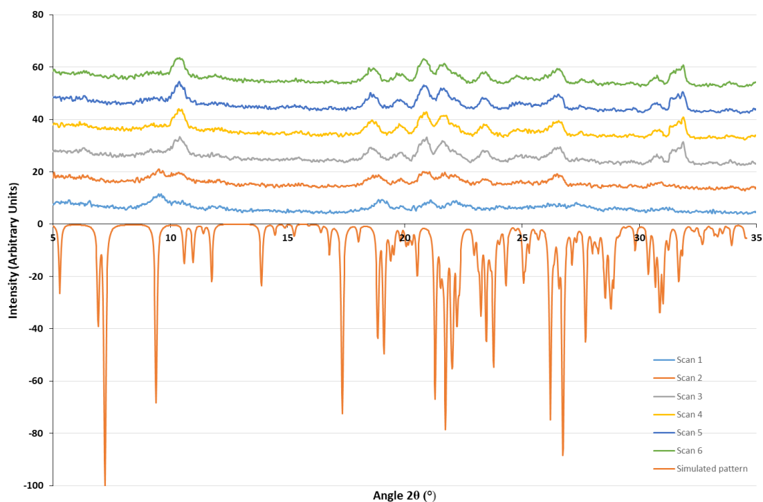
Figure 2.16 Time course X-ray powder diffraction of 62 collected immediately after removal from the recrystallisation solvent, showing the rapid loss of the original poorly-crystalline phase and growth of the collapsed microcrystalline phase. Each of the scans 1 – 6 corresponds to 3 minutes exposure. The dry sample was measured after drying the sample in vacuo with a 30 min exposure time. The simulated pattern was obtained from the X-ray data.
