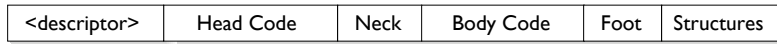
Figure 4.2: In the OPAM, a clause is encoded into a descriptor called the clause descriptor record , head code, neck, body code, foot and the code size, followed by structure sequences.
