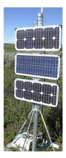
Figure 5.5: Deployed Village DTN Router. This is the router shown at Sallohaure during the trial in summer 2010. One can see the stand, 3 x 20W solar panels, infrastructure-mode WiFi antenna (cropped at the top of the image) and the enclosure (at bottom) containing the electronics.
