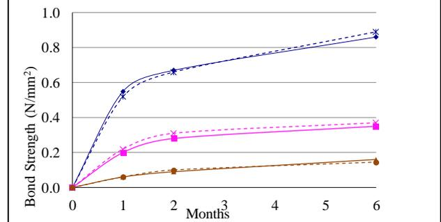
Figure 9 Bond strength of masonry cured outdoor over time
