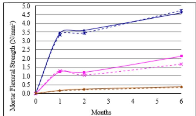
Figure 8 Flexural strength of mortar cured outdoor over time
