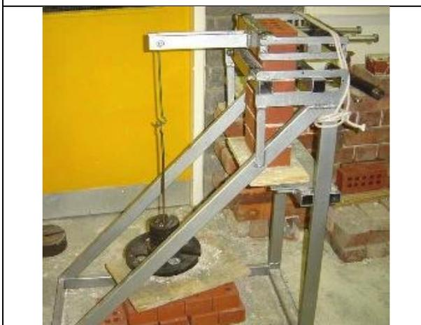
*Fig.3 Bond strength test set up.*
