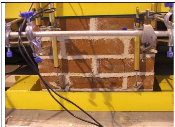
*Fig.2 Compressive strength masonry test set up.*
