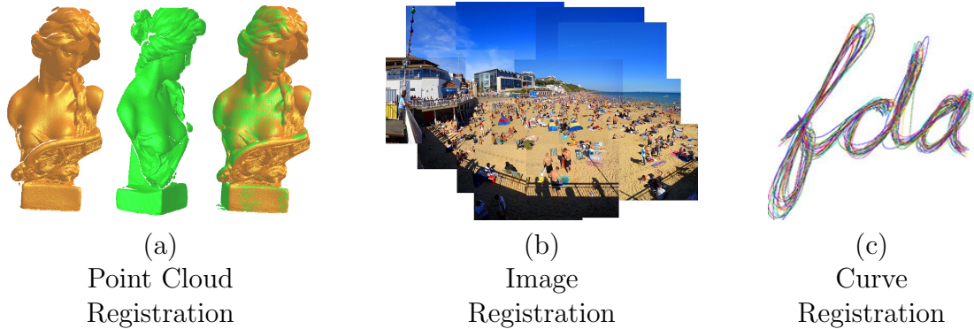
Figure 1.2: Applications of shape registration. (a) Point cloud registration: the meshes shown in gold and green (left) are registered so that they are aligned (right); (b) Image registration: several images of the same scene are registered to create a larger picture of the scene; (c) Curve registration: several curves representing the letters ‘fda’ have been registered so that they overlap.
