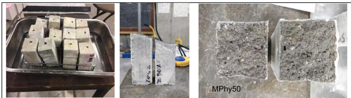
Fig. 3: Water Absorption test
