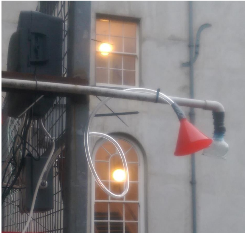
Figure 5.6 Collocated inlets of sensing node (red funnel) and DCC fixed site monitors (clear plastic) at Coleraine st.
