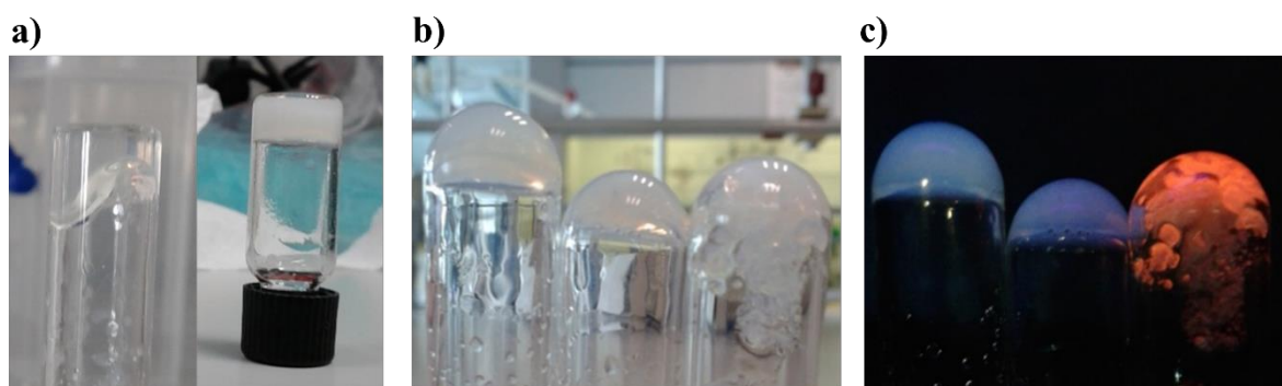
Figure 2.24 Optical images of a) ligand hydrogels formed from 120(S,S) at 6 wt% (left) and 10 wt% (right) showing transparent and opaque materials, respectively; b) ligand hydrogels of 120(S,S) at 6 wt% (left), 10 wt% (middle) and 5 wt% Eu III -doped (right) under ambient light and; c) the same hydrogels in b) under UV light ( \lambda_{\text{exc}} = 254 nm).
