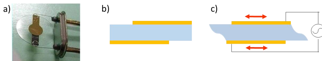
Figure 2.12. (a) Picture of a 10 MHz QCM sensor and a schematic representation of the quartz crystal with the gold electrodes on each side (b) before and (c) after applying the external driving oscillating circuit.
