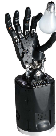
Figure 2.20: Shadow Dexterous Hand C6M gripping a light bulb (taken from [64]).
