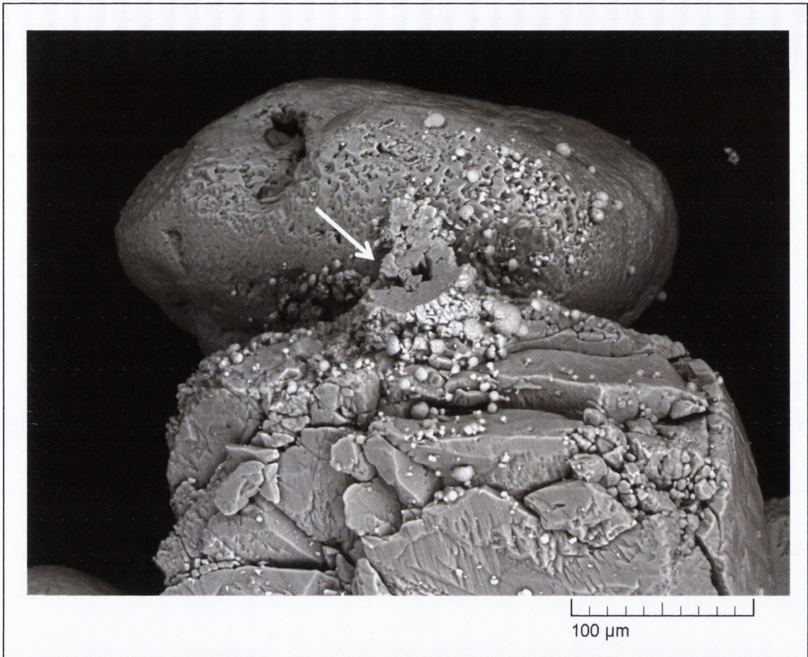
Figure 5.14 Detail of a carbonate structure bonding three silica sand particles after eutrophic treatment. The arrow indicates where a detached particle left behind a smooth concave imprint (sample EE1).
