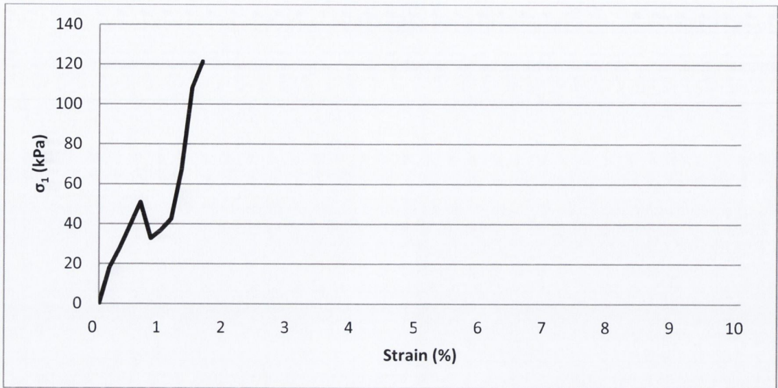
Annex 31 Sample E500 UCS (wet) stress-strain curve. Data beyond the point of failure could not be recorded due to the complete collapse of the sample.
