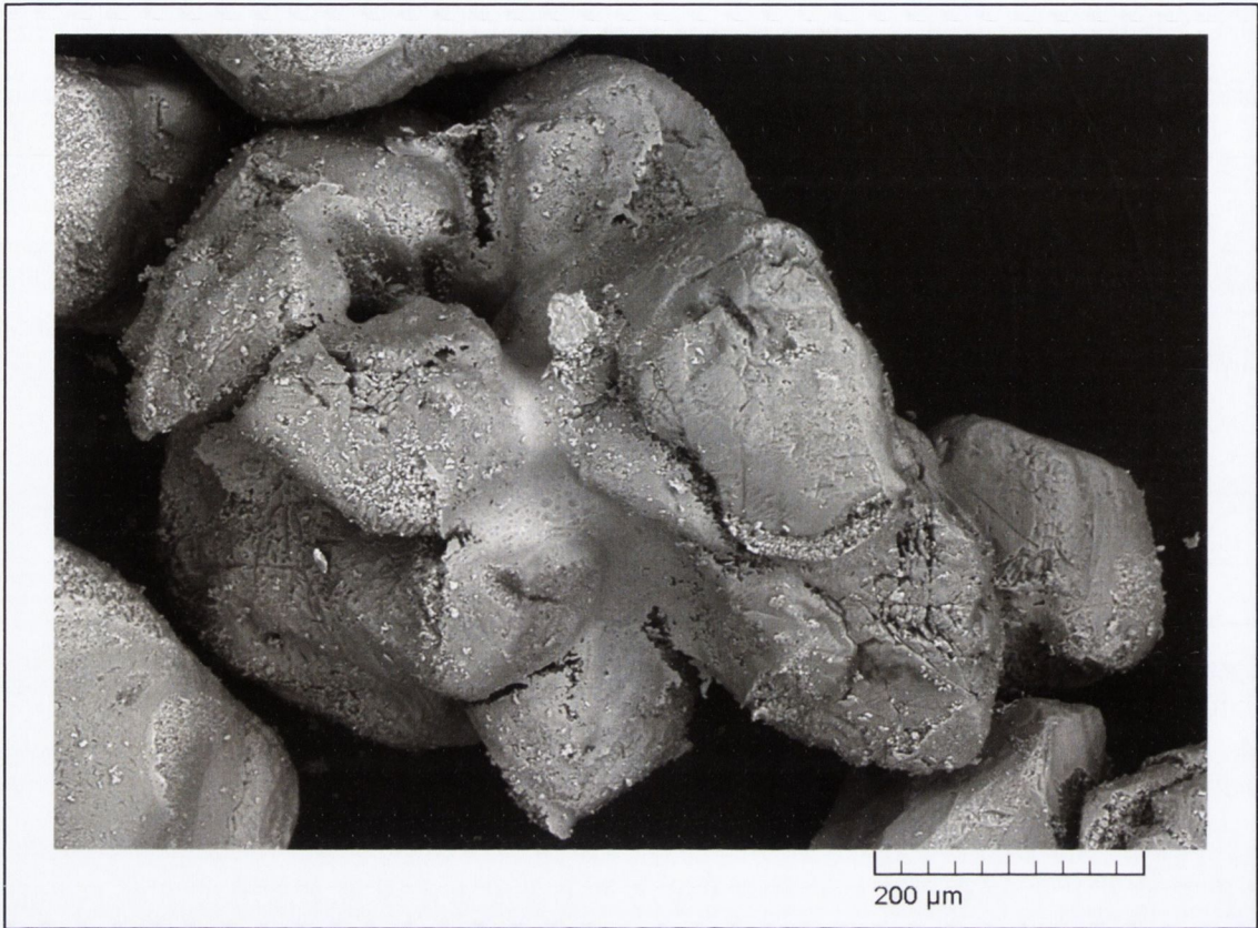
Figure 6.8 Cluster of sand particles held together by calcium carbonate bonds formed during the atomised delivery of cementing agents (sample E150). The calcium carbonate precipitated traces the shape of water menisci formed during the reaction time.
