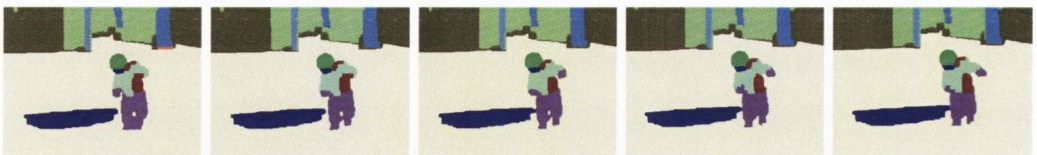
(b) Label propagation results using the \alpha -expansion method [16]. In segmentation result of central frame, label of pixel belonging to the left hand (left glove) of the boy is different from the previous frame. Label of segment representing the trouser is assigned to those pixels. Temporal consistency metric penalize the segmentation for this change (Figure 6.9).
