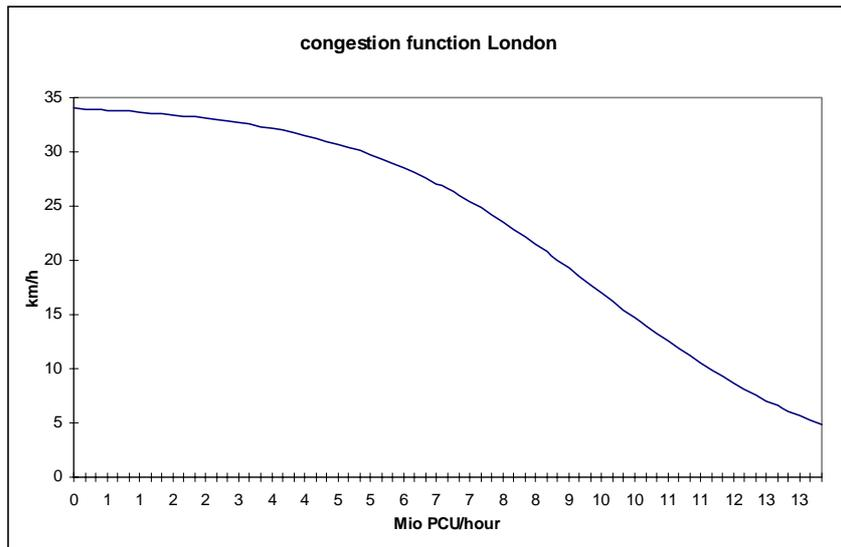
**Figure 3** Speed-flow relationships for a car in the interregional model
