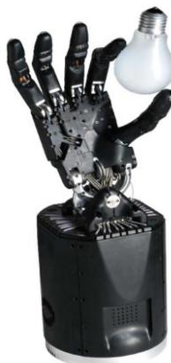
Figure 2.1: Shadow Dextrous Hand C6M [3]
