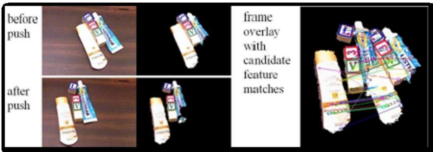
Figure 3.1: Interactive Singulation of an Object from a Pile [23]
