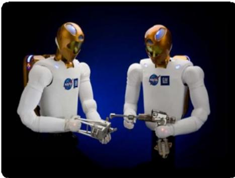
**Figure 2.2: NASA Robonaut 2 [8]**
