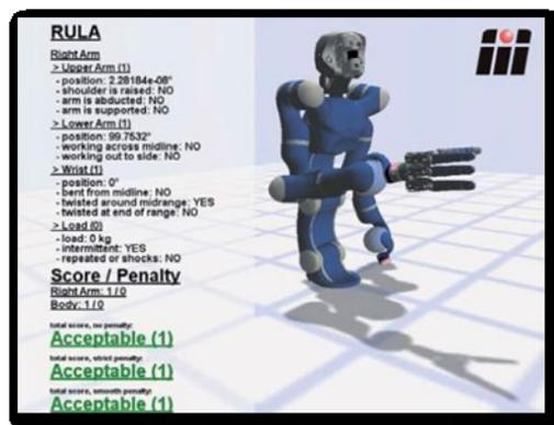
Figure 4.1: Using the RULA Evaluation Criterion to Determine Natural Poses [31]
