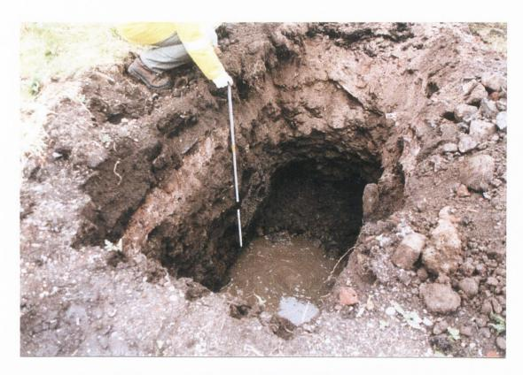
Figure 4-14: Trial pit (TP3) excavated in the vicinity of load tests
