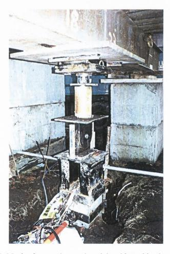
Plate 3-10: Mechanism used to apply axial and lateral loads to pile AL1
