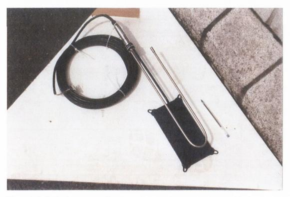
Figure 3-5: Typical pressure cell
