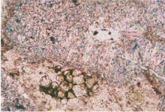
Figure 6. Petrographic micrograph of Howth Harbour mortar with remnants of unhydrated clinker (cluster of alite, belite and dark interstitial phases) and secondary  $\text{CaCO}_3$  filling fracture (top) 40X polarized light.
