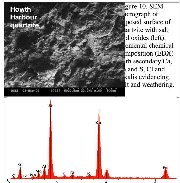
Figure 10. SEM micrograph of exposed surface of quartzite with salt and iron oxides (left). EDX elemental chemical composition (EDX) showing secondary Ca, Fe and S, Cl and K evidencing salt and weathering.
