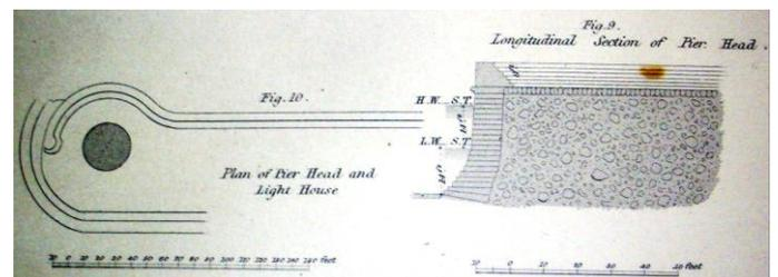
Figure 4. Rennie’s section and plan of the East pier, constructed with the diving-bell.
