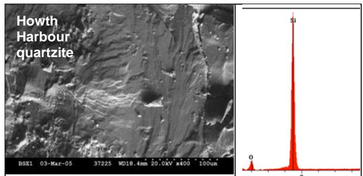
Figure 9. SEM micrograph and EDX analysis of quartzite at c. 10mm depth consisting of unweathered pure quartz.
