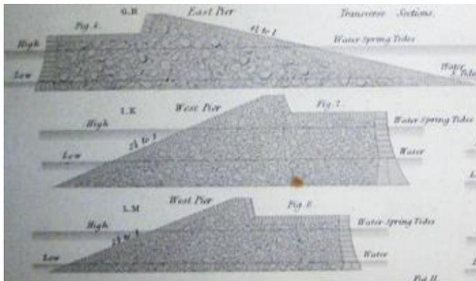
Figure 1. Rennie’s sections through the slant piers (East and West), built à pierre perdue before the introduction of the bell.
