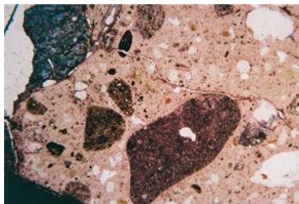
Figure 5. Petrographic micrograph of Howth Harbour mortar with coarse dolomite (left) and limestone aggregate, in a fractured, largely carbonated binder. 2X polarised light.
