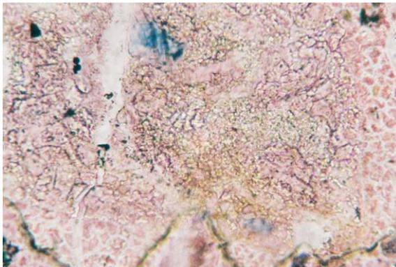
Figure 7. Calcium silicates and CSHs in a Harbour mortar 40X natural light.
