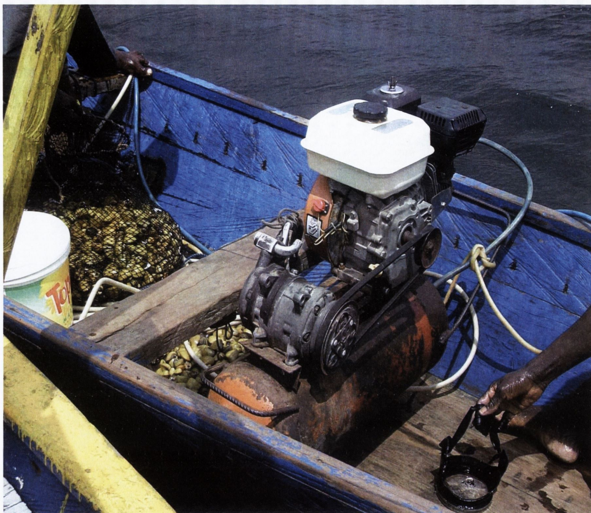
Figure 2.3 Hookah fishing accessories (compressor, mask and net bag) used for clam fishing in the deeper zones at Ada and Aveglo by young men at the Volta Estuary.
