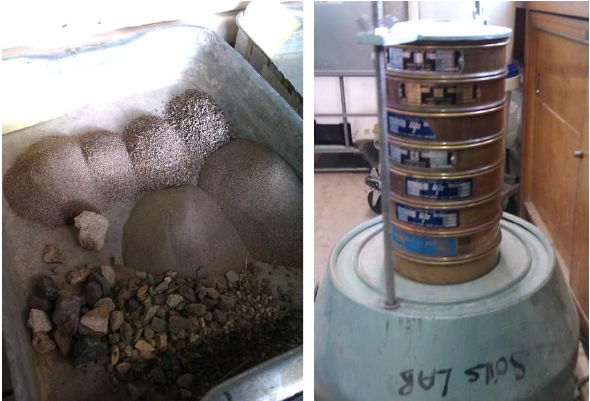
Figure 4.17 (a) A fully sieved sample from Carrigeen, Co. Kilkenny showing quantities passing the different sieves (b) A full stack of sieves from 2.0 mm down to 0.063 mm
