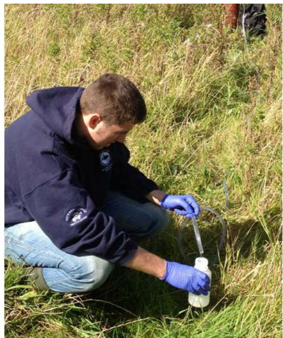
Figure 4.12 (a) Waterra WaSP-P3 Pump (b) Sample being taken using the Waterra pump
