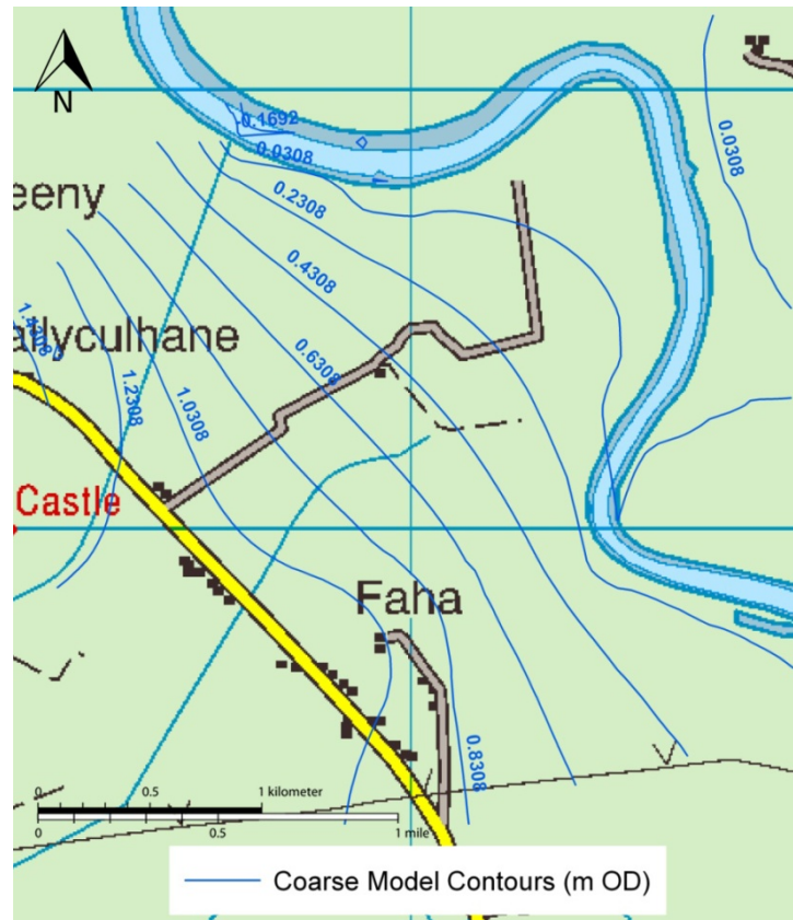
Figure 8.18 Modelled groundwater contours at Faha, Co. Limerick
