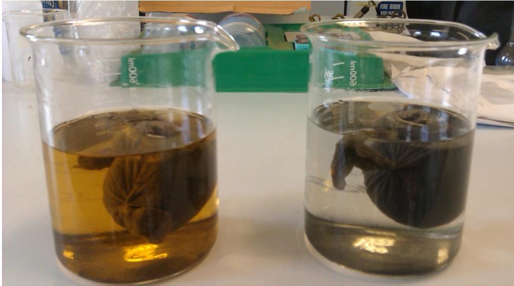
Figure 5.52 Charcoal Bags located downstream (left) and upstream (right) showing tracer removed by eluting solution
