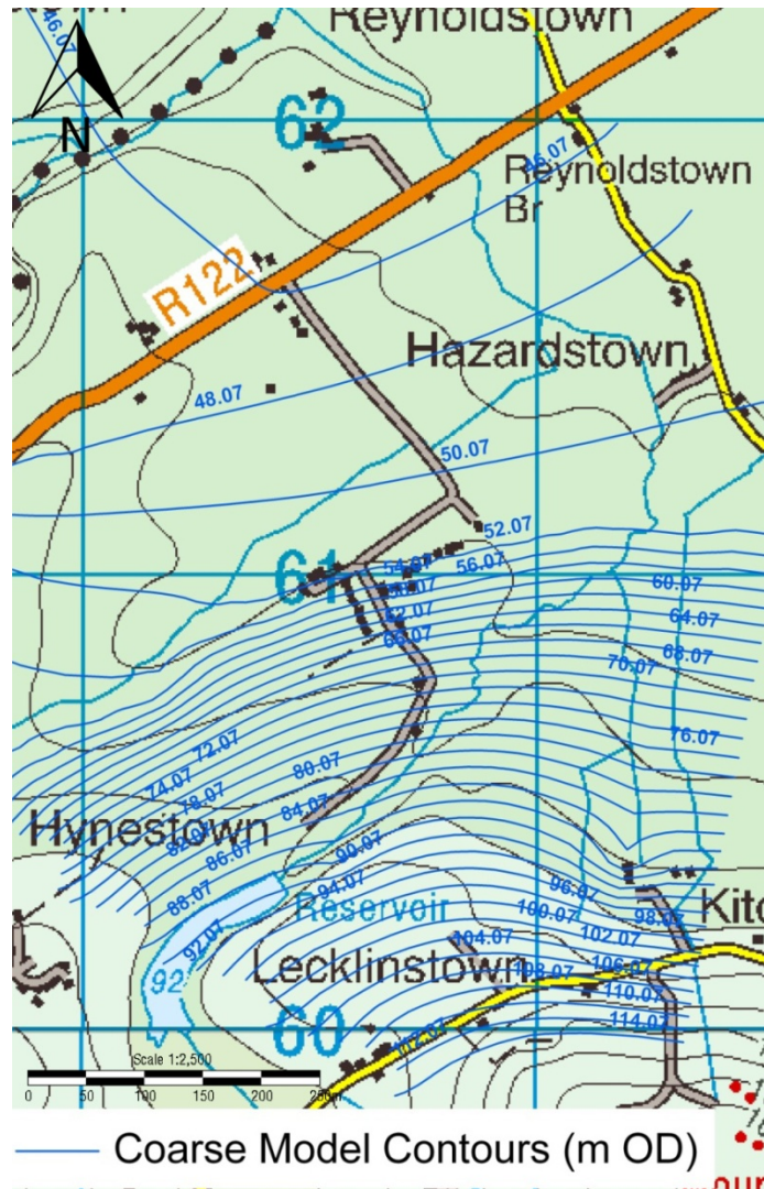
Figure 8.14 Modelled groundwater contours at Naul, Co. Dublin
