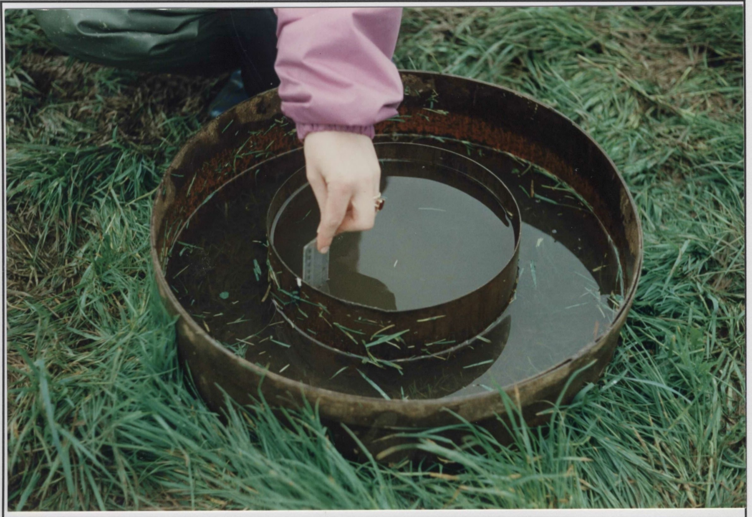
Plate 4.7 Double ring infiltrometer used to measure soil infiltration capacity.
