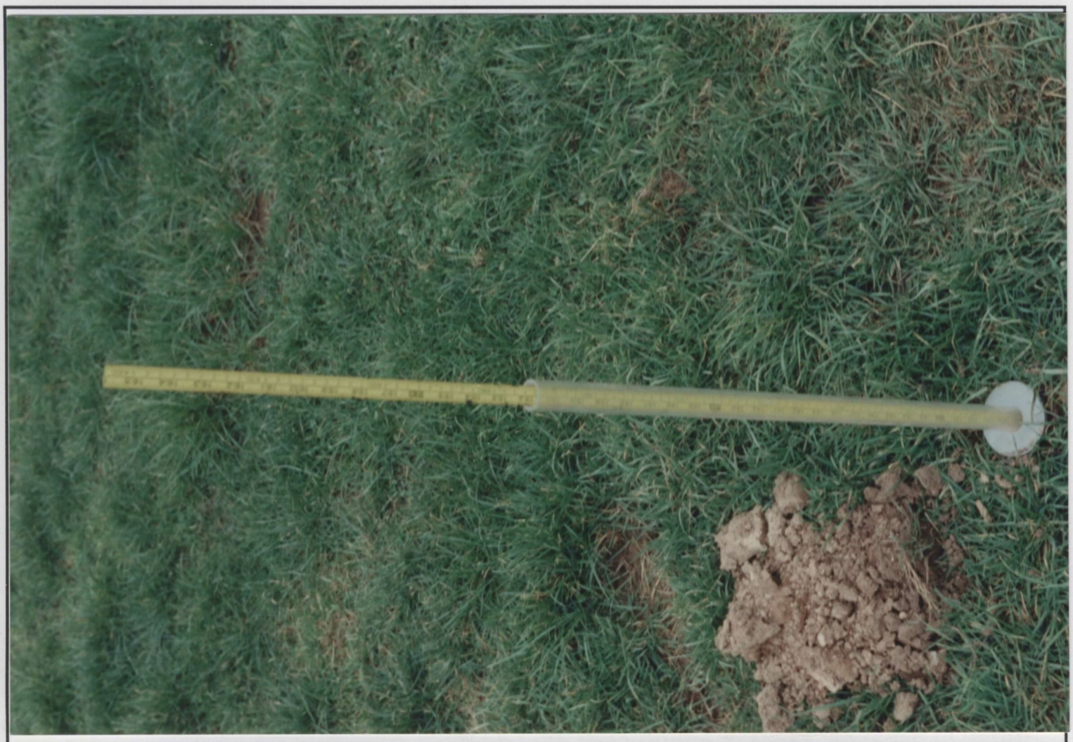
Plate 4.8 Inversed auger-hole method for Quaternary deposit permeability measurement.
