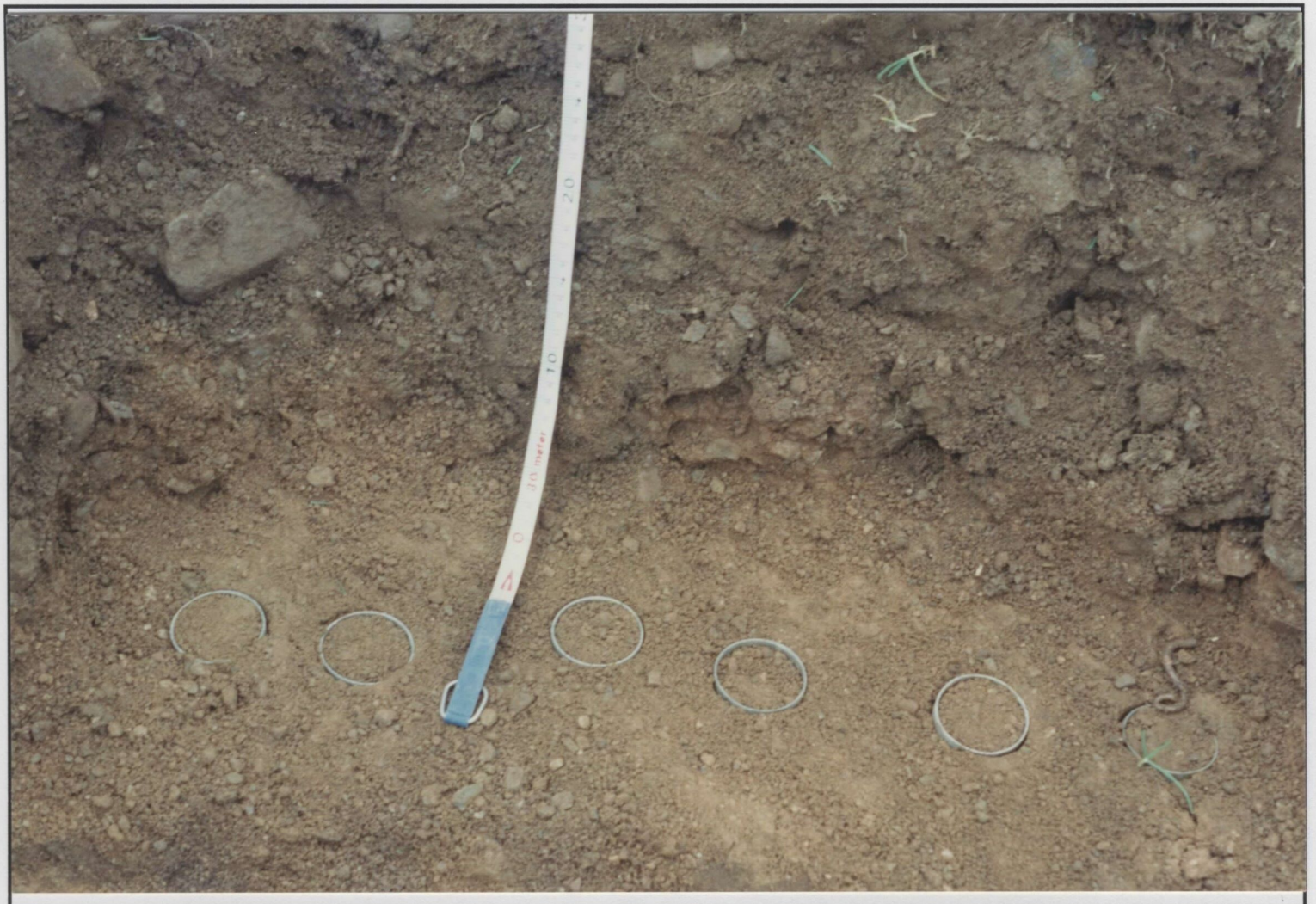
Plate 4.6 Six soil cores in trial pit taken for bulk density determination.
