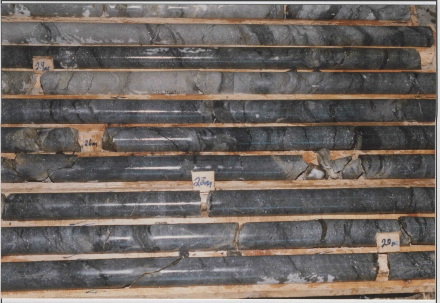
Plate 5.4 Ballysteen limestone between 20 and 30 m of the bedrock core in borehole 5. Solutionally enlarged bedding partings observed. Cores decrease in depth from the base of the photo to the top and from right to left.
