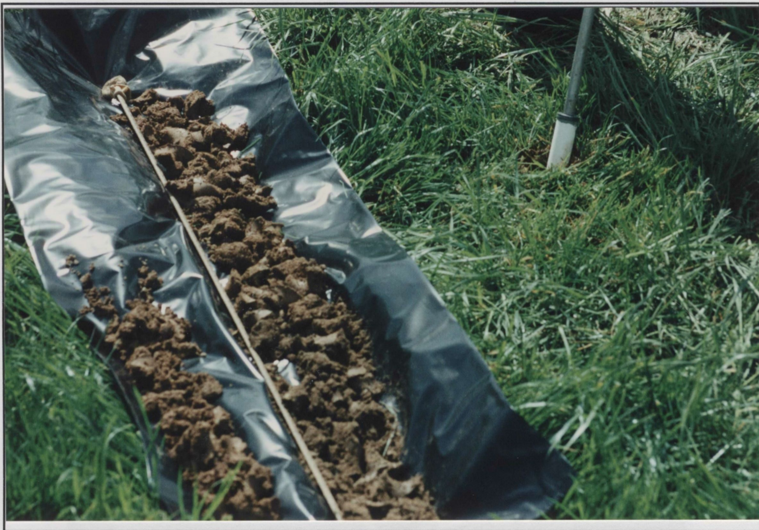
Plate 6.1 Field insertion of a ceramic cup being pushed into an augured hole. The stratigraphic sequence of soil removed from the hole can be seen to the left of the photo.
