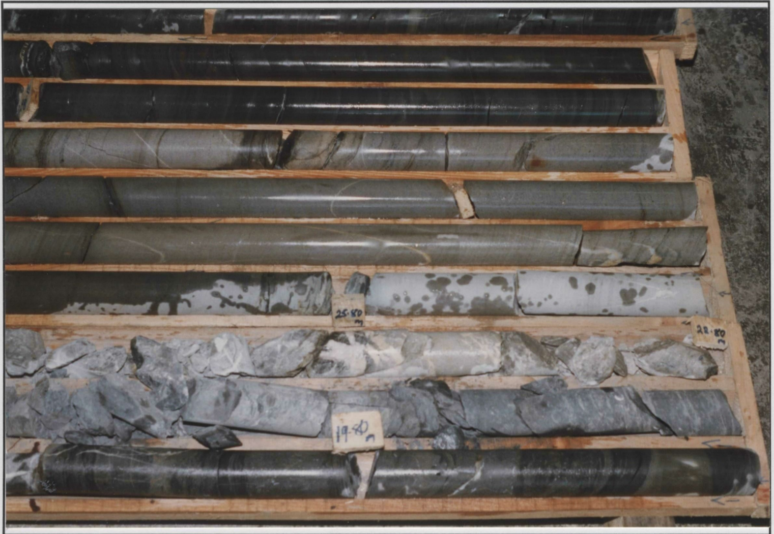
Plate 5.2 Fault area of bedrock core (fragmented area at bottom of photo) from borehole 4, with grey Ballyderown sandstone above the fault (after 25.8 m tag). Cores decrease in depth from the base of the photo to the top and from right to left.
