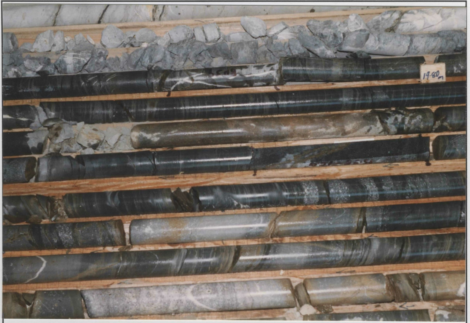
Plate 5.1 Ballysteen limestone bedrock core in borehole 4, cores decrease in depth from the base of the photo to the top and from right to left.
