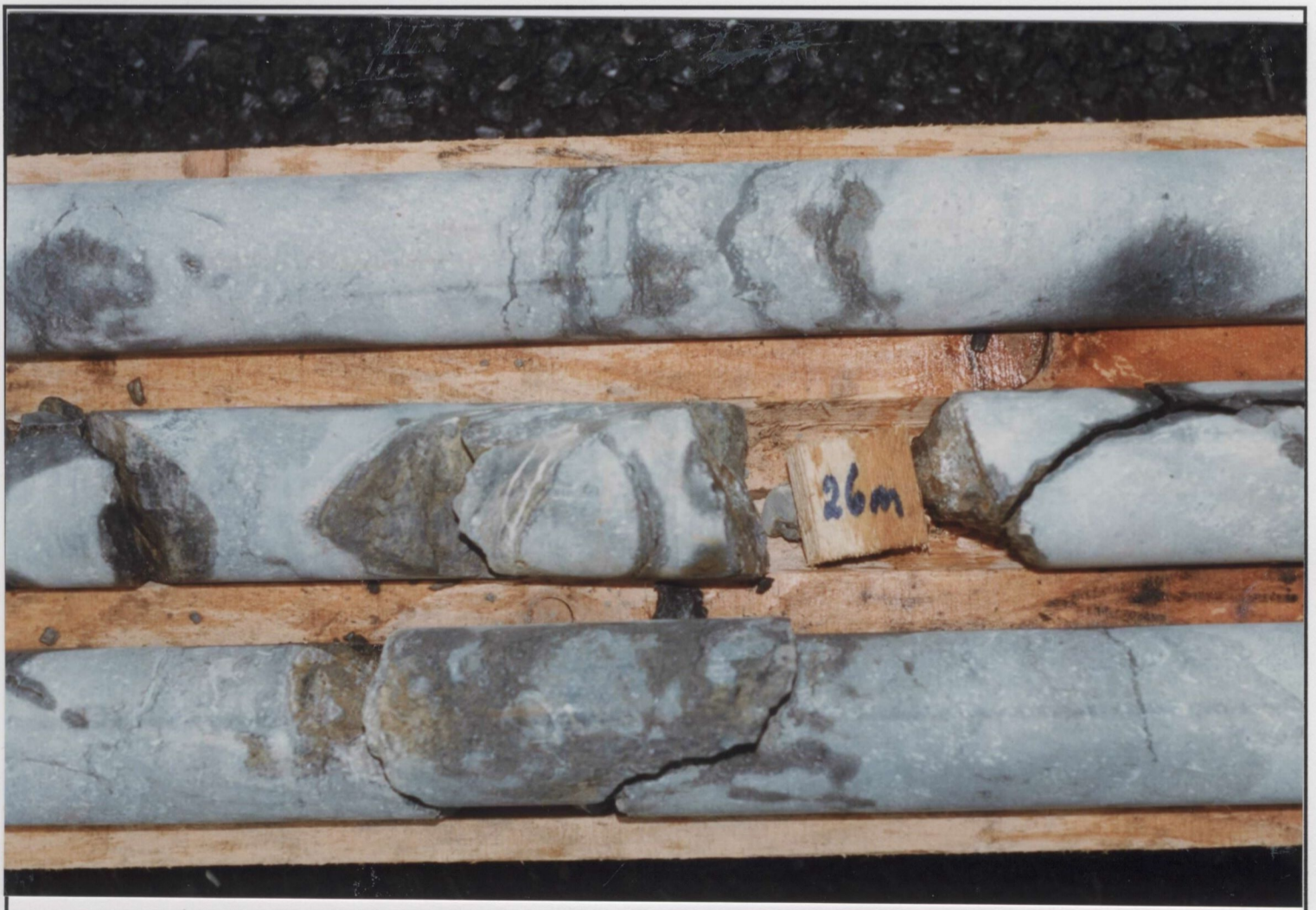
Plate 5.5 Solution of limestone bedrock at a depth of 26 m b.g.l. in borehole 5.
