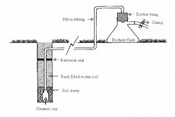
Figure 6.7 Schematic insertion of a ceramic cup.
