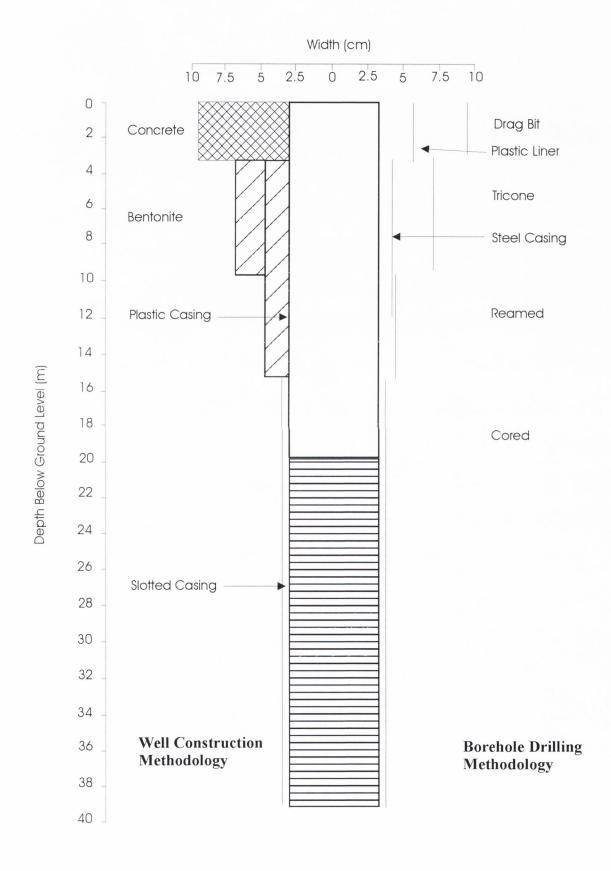
Figure 5.1 Borehole drilling methodology and monitoring well construction.
