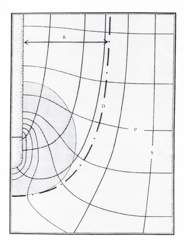
Figure 6.1 Potential field around a suction cup in a homogeneous soil (R, radius of the recharge area; D, dividing stream line; P, iso-potential line; S, stream line; dotted field, space from which the sample is taken.)
