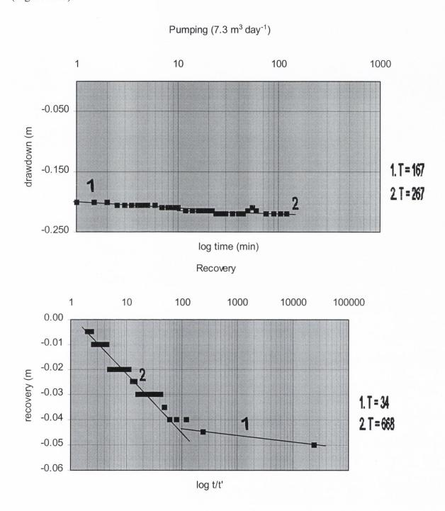
Figure 5.10 Pumping and recovery graphs for borehole 5, in 1994, showing the straight lines used for calculation of transmissivity values, T values for each line are presented (m<sup>2</sup>day <sup>-1</sup>).
