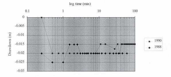
Figure 5.8 Draw down observations carried out in borehole 1 in 1988 (Q=6.5) and 1990 (Q=5.4).
