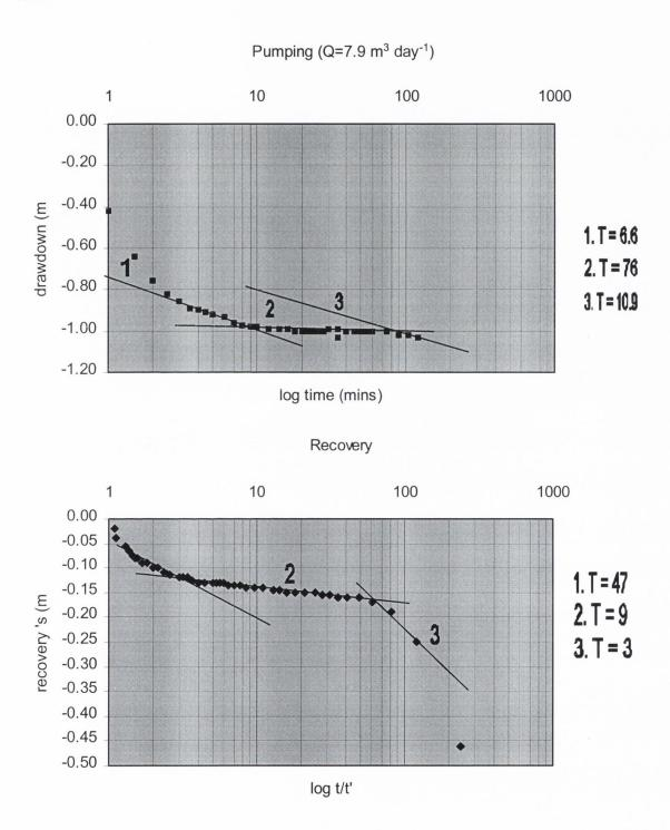
Figure 5.9 Pumping (Q=7.9 m³ day⁻¹) and recovery graphs for borehole 4, in 1994, showing the straight lines used for calculation of transmissivity values, T values for each line are presented (m²d⁻¹).
