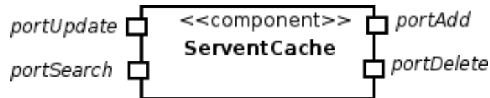
Fig. 6.4: A UML diagram presenting a conceptual view of the ServentCache component.
