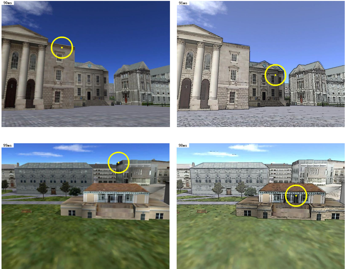
Figure 4.1: Example of two scene images with and without abstraction. The yellow markers indicate the most salient points of each image, as indicated by the saliency metric, described in [IKN98]. In each stylised image the most salient point is found to be the object which is focused on using adaptive abstraction. The right images use the Kuwahara filter, difference of Gaussian edges and saturation variation. These images show that the most salient point can be changed by using our adaptive abstraction approach.
