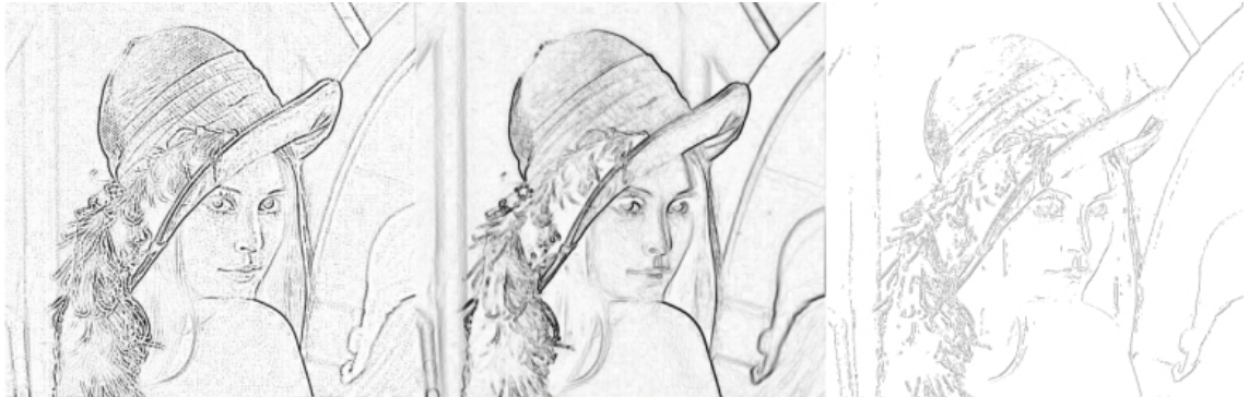
Figure 3.2: Edge detection examples; Difference of Gaussian (Left), Sobel (Centre), Canny (Right)
