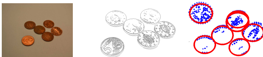
Figure 7.17: Examples of detecting ellipses in RGB images.
