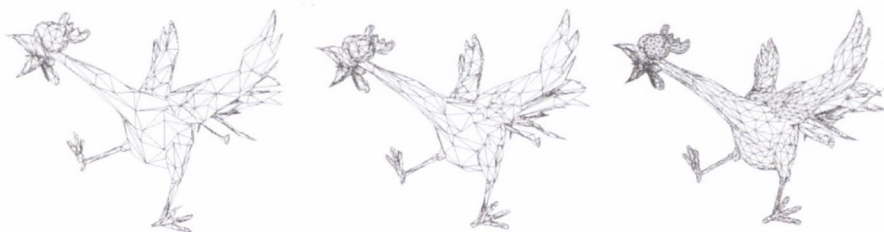
Figure 2.5: 3D mesh representation using different resolutions (increasing the number of faces) [3].
