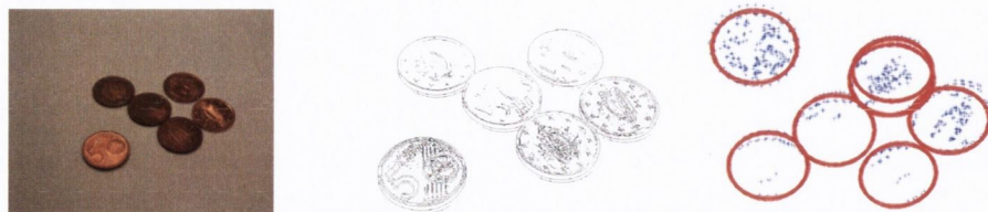
Figure 7.17: Examples of detecting ellipses in RGB images.
