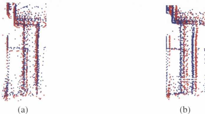
Figure 5.21: Details of the alignment between buildings. a) using our proposed algorithm for aligning the scans and b) using ground truth.
