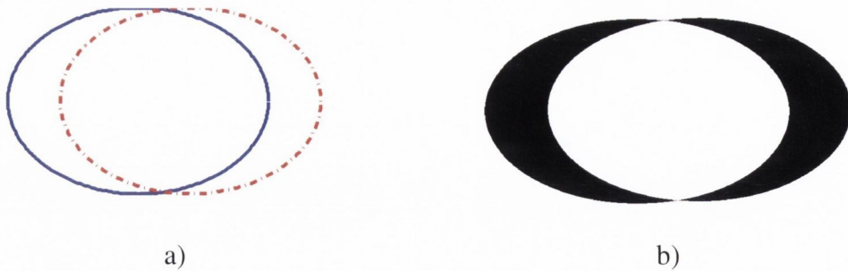
Figure 7.6: Example of computing the error rate. Figure a) shows in blue the true ellipse (observation) and in red dots the estimated one. The black region in figure b) represents the area of the symmetric difference in between the two ellipses.
