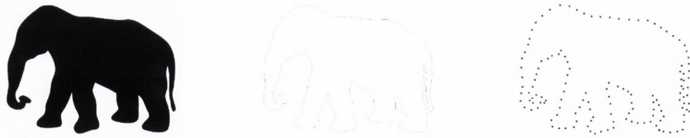
Figure 2.3: Point Cloud description by sampling the edge image.
