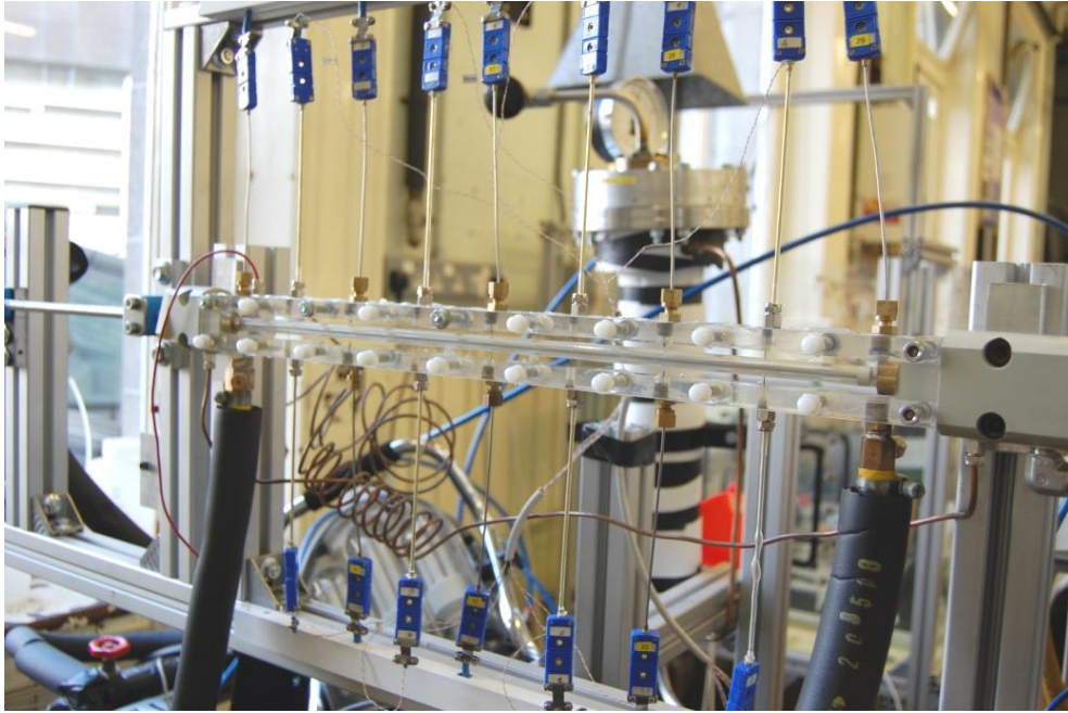
Figure 31: Test section showing developing length, sapphire tube, perspex jacket and polypropylene support pieces
