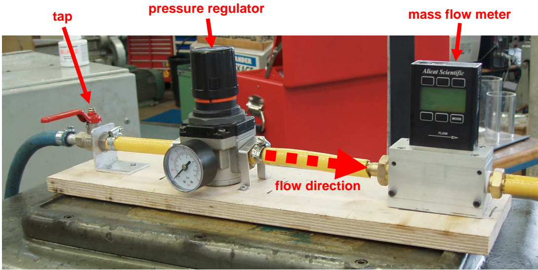
Figure 18 – Pressure control and flow rate measurement station: pressure regulator and mass flow meter
