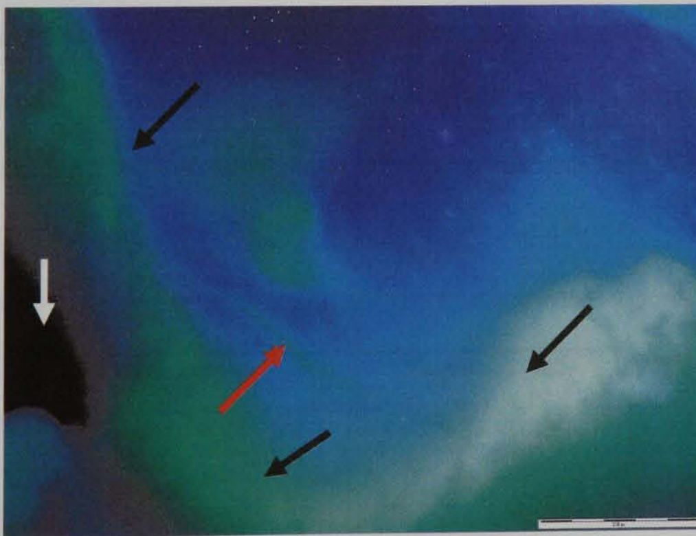
Figure 2.9 Oxytetracycline diffuse stained area (Black arrows) and one microcrack (Red arrow) examined using epifluorescent microscopy using UV light (365 nm). A white arrow indicates the implant. Scale bar = 50 \mu\text{m} .
