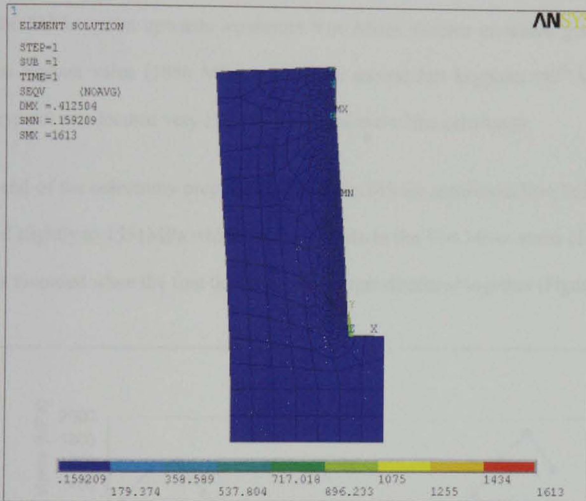
Figure 3.9 Maximum Von Mises stresses when the keypoint no. 1, 4, 7 and 10 were displaced. The maximum Von Mises stress (1613MPa) was located close to the displaced keypoint number 10. A lower stress (717MPa) could be observed around the 1 st keypoint and 358MPa around the 4 th keypoint. The predicted stresses were presented in Mega Pascal units (MPa).
