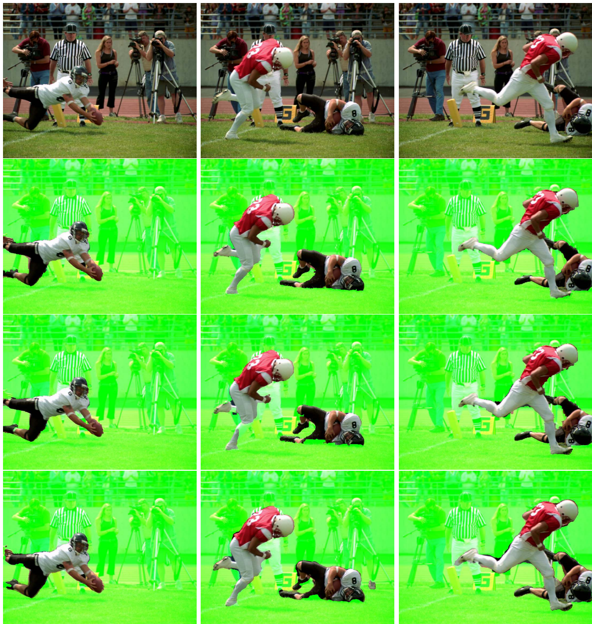
Figure 8.8: The foreground/background level segmentations for three frames in the Artbeats-SP128 sequence. The foregrounds are extracted using the respective segmentations and the backgrounds are shaded in green. Top row: Frames 20, 62 and 95 in this sequence. Second, third and bottom rows: The segmentations for the frames in the top row produced by our Semi-Auto , Geodesic and the NUKE approaches respectively.
