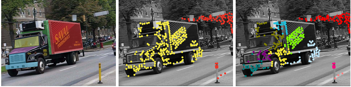
Figure 2.10: Left: A truck shown at frames 1 in a motion sequence from the Hopkins dataset [117] available online. Some roughly planar surfaces on the truck are highlighted in red, green, yellow, purple, and cyan. Center: The desired labels for a 3D segmentation technique. The points along the trajectories for the background and truck are red and yellow dots respectively. Right: The trajectory segmentation result produced by our proposed sparse segmentation technique. Each trajectory bundle shown in a different colour roughly represents a single surface of the truck.
