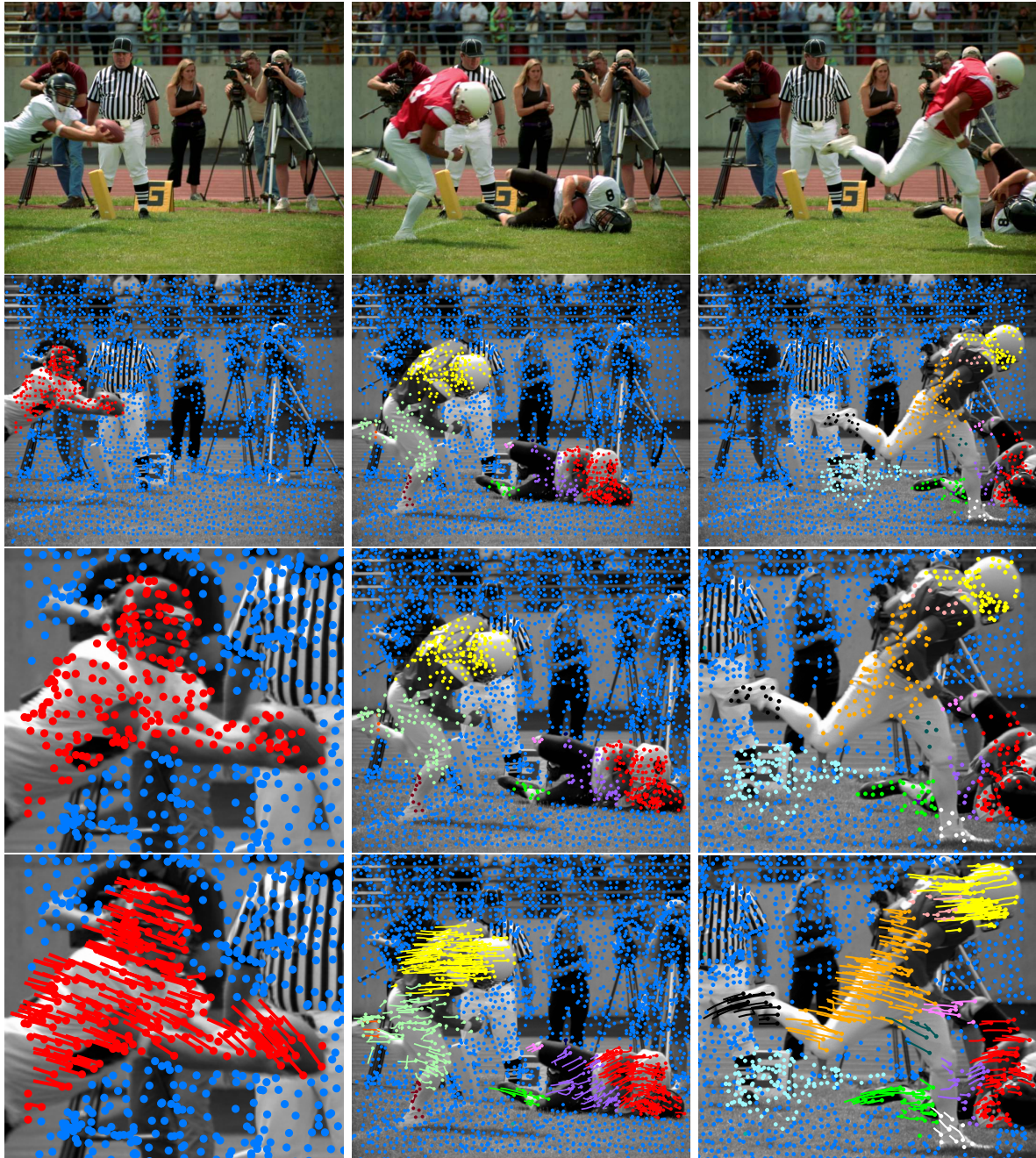
Figure 6.18: Top row: Frames 3 (left), 57 (center) and 98 (right) in the Artbeats-SP128 sequence. This sequence is a scene from an American football game. The foreground objects here are player #1 and #2 in red and white jerseys respectively. Second row: Our segmentation for the frames in the top row. Here the trajectory points for the background bundles are cyan and blue dots. All the other trajectory bundles represent player #1 and #2 in the foreground. Third and bottom rows: A zoom on the trajectory bundles corresponding to the players. The third row shows the points of the trajectories at the current frames, while the bottom row shows the motion history of each trajectory up to the current frames. For clarity only the motion history over the last 5 frames is shown for each trajectory.
