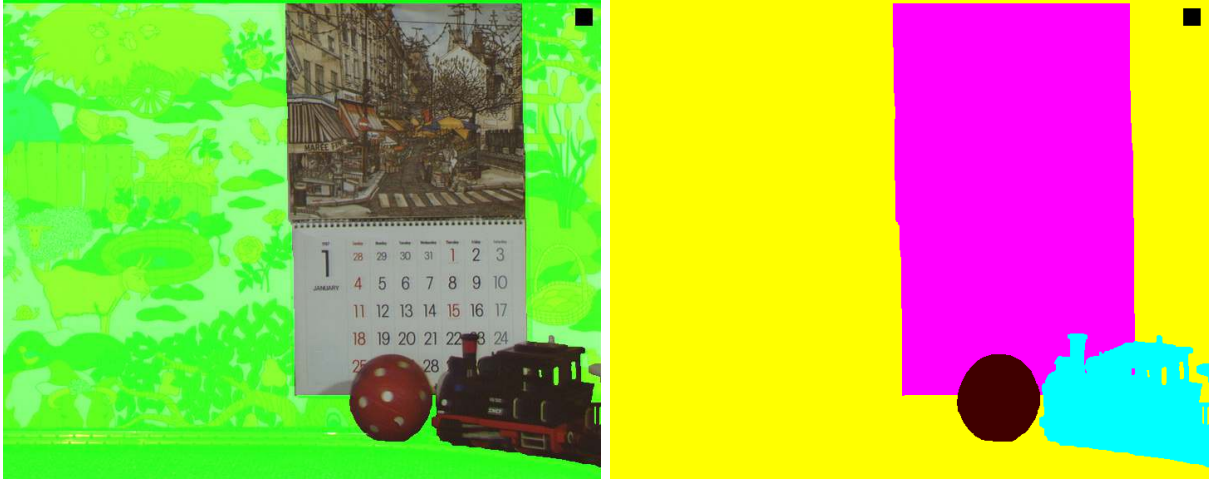
Figure E.2: The key frame for frame 1 in the Calendar and Mobile sequence. The foreground on the left is extracted using the key frame on the right where foreground is any colour that is not yellow (background). Both these representations are indicated as key frames by the black squares in the top right corners.
