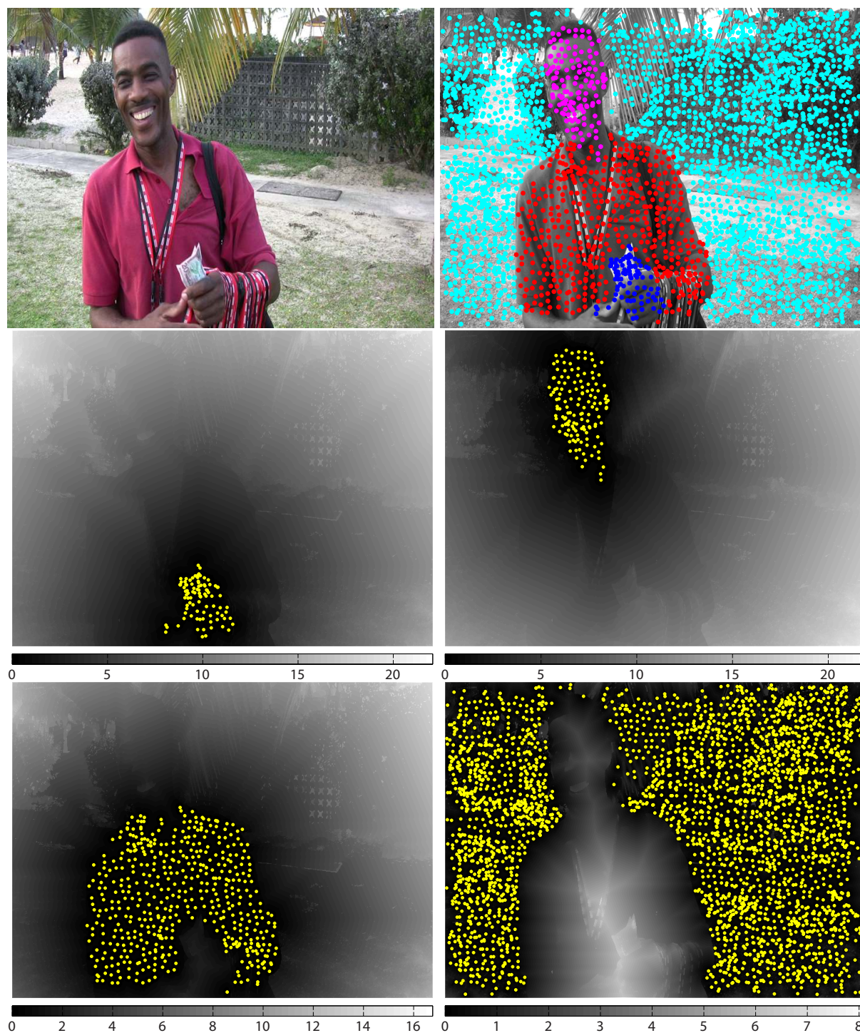
Figure 7.8: The geodesic distances to the objects in frame 2 of the Triniman sequence. Top row: Frame 2 (left) in the Triniman sequence, and our sparse trajectory segmentation (right) for this frame. The points for the trajectories shown as coloured dots. The four trajectory bundles are coloured cyan (background), pink (face), red (body) and blue (hand) respectively. Clockwise from middle left: The geodesic distance to the hand, face, background and body objects respectively. The respective points of the trajectories are superimposed on the geodesic distance fields as yellow dots. The values for the geodesic distances are represented in gray scale, where black and white are minimum and maximum values respectively.
