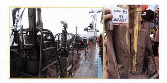
Figure 3.13: Box corers used in GLOW Box coring and sediment retrieved via plastic liners with way-up indicators (arrows) marked on the tubes (GLOW Survey Team).
