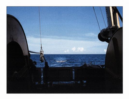
Figure 3.3: Submerged sleeve guns immediately after shooting and streamer cables from stern of the Pelagia., GLOW Survey 2009.
