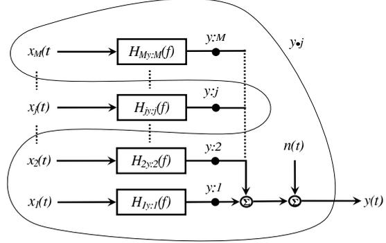
Figure 1. Multiple Source Acoustic Measurement
