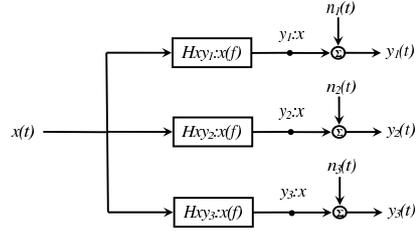
Figure 3. Signal Enhancement Model
