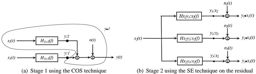
Figure 4. Conditional Spectral Analysis Technique
