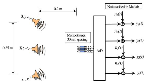
Figure 5. Schematic of the Test Set-up
