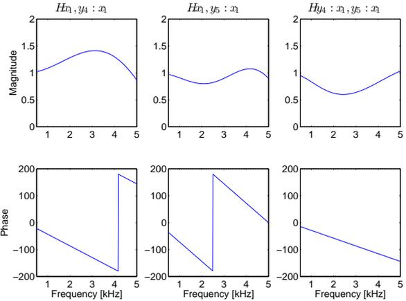
(b) Transfer functions as a result of using FIR1 filters
