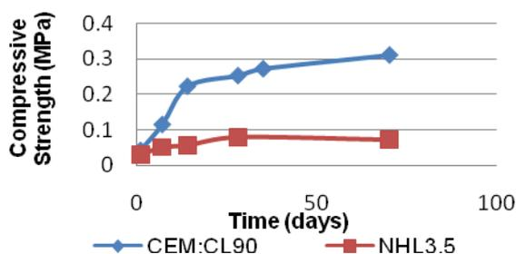
Fig. 1: Strength development of the concretes over time.
