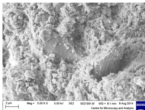
Fig. 5: SEM image of NHL3.5 binder at 1 month including significant hydrates and carbonates.
