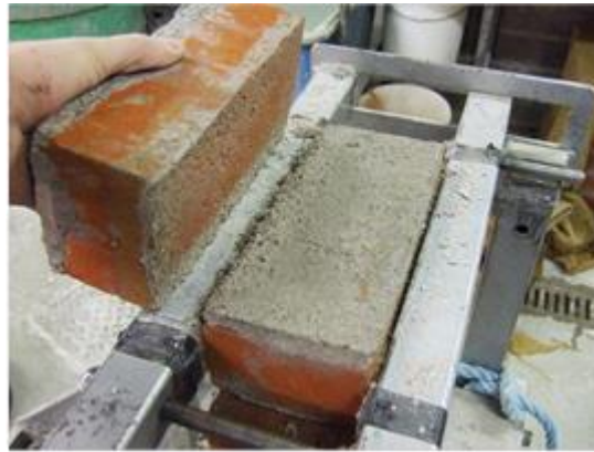
Figure 4. Flexural bond wrench test failure at the mortar interface with the upper unit (A1 mode)
