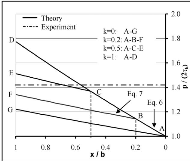
Figure 4. ECAE vertical stress distribution(10x10)
