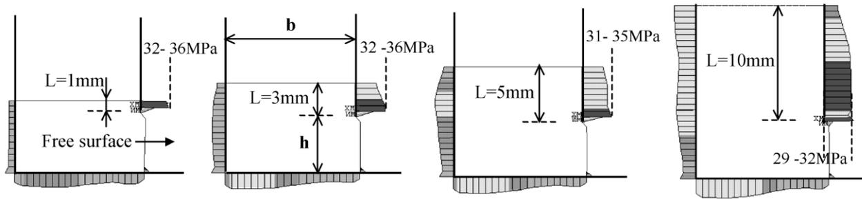
Figure 9. Tool stresses from a Finite Element Analysis
