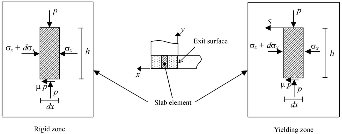
Figure 3. Stress system in the intersection zone
