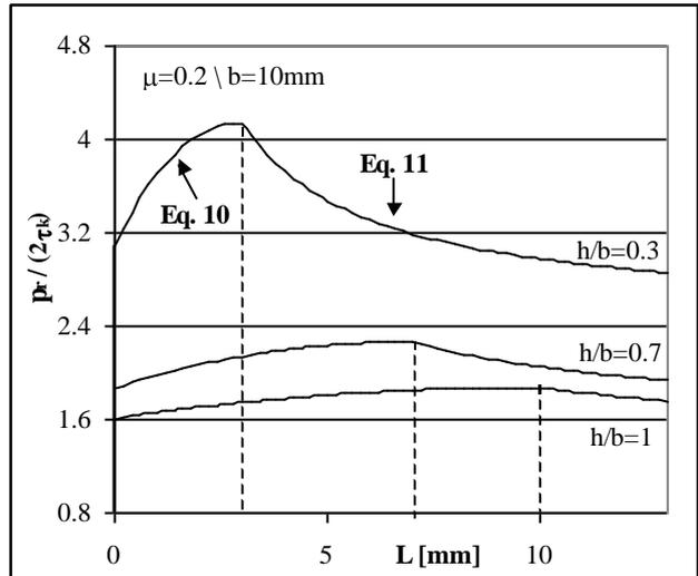
Figure 8. Pressure on the right hand side wall
