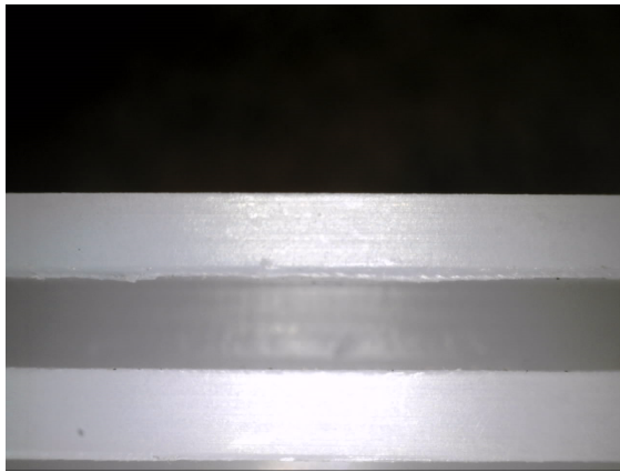
(a) Sharp tool, showing smooth surface and no deformation
