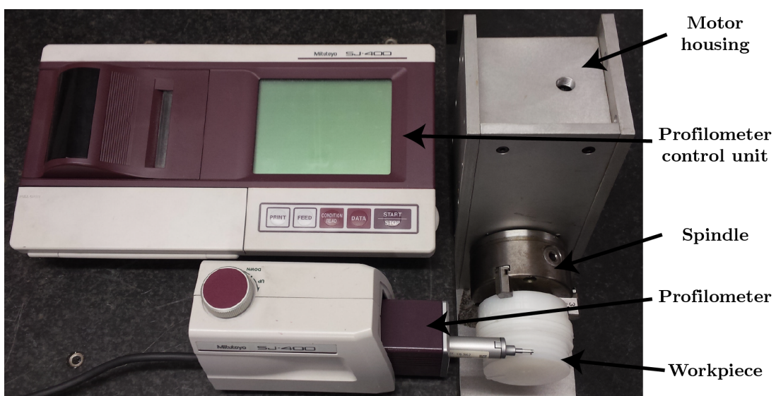
Figure 3.5: Profilometer and spindle setup for measuring surface roughness on round parts. Not shown: Laptop used for control and data acquisition.
