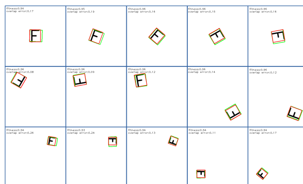
Figure 5: Examples of matching results. Red rectangle represents the ground true, green rectangle represents the matching result.
