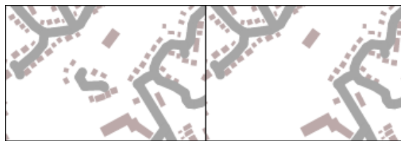
Figure 3: Fix step applied to floating roads. Before (left) and after (right).
