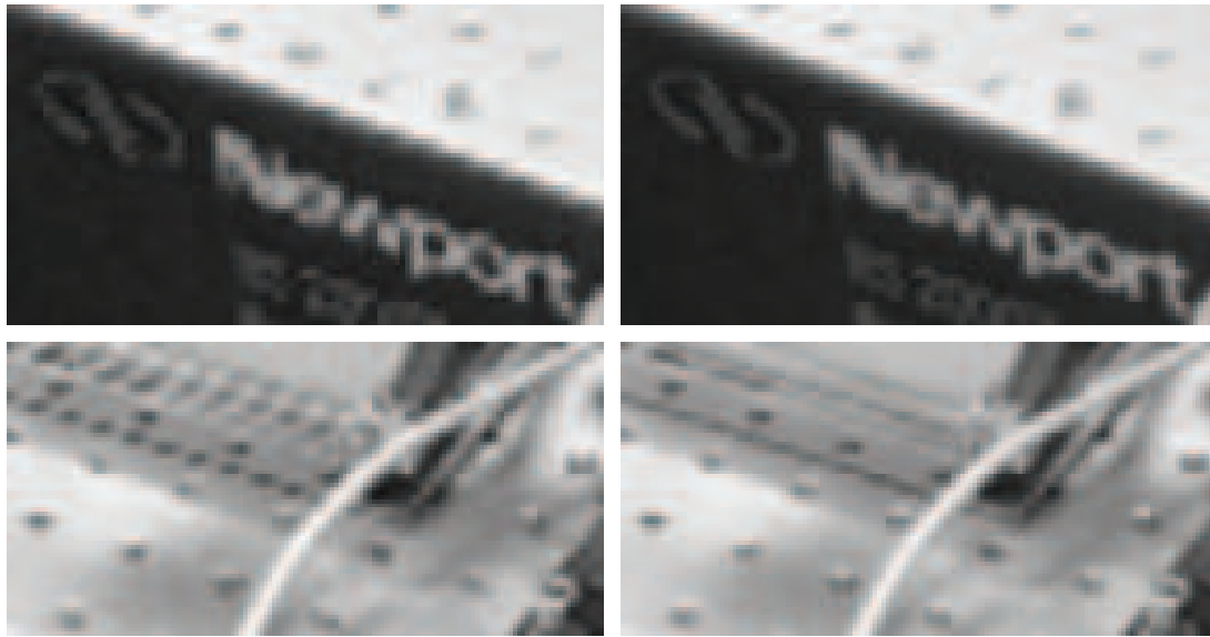
Figure 2: Comparison of super-resolution results applied to simulated low spatial frequency images. (left) images obtained through Sinc interpolation of input images, (right) results of super-resolution. Sharp discontinuities across edges and periodic gradients are visible in the interpolated output. Upon application of super-resolution, more continuous detail is visible along edges. The input sequence for the super-resolution process was 23 randomly shifted images.
