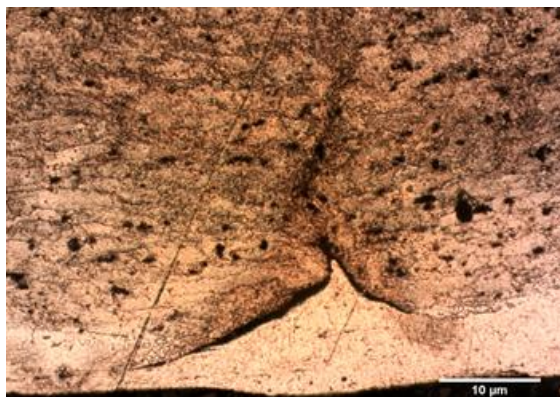
Fig. 4 Remnants of joint line at the bottom of the weld produced by tapered cylinder
