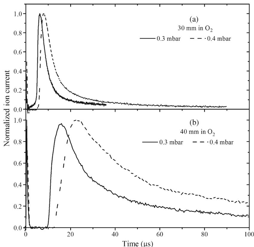
**Figure 3.** Ion currents measured using a planar Langmuir probe placed at same positions of substrates, (a) 30 mm and (b) 40 mm. FWHM are (a) 4 and 6  $\mu\text{s}$  and (b) 16 and 31  $\mu\text{s}$  for 0.3 and 0.4 mbar of  $\text{O}_2$ , respectively.
