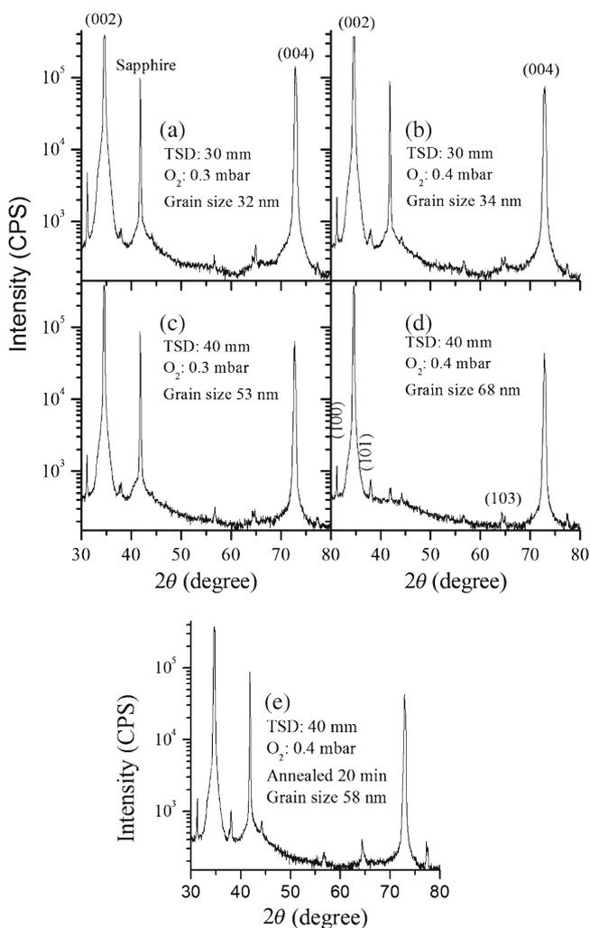
**Figure 1.** XRD pattern of *c*-oriented ZnO films and corresponding grain size, as calculated using Scherrer formula, together with growth parameters. Figures (a–d) correspond to as-grown films while figure (e) corresponds to a film annealed for 20 min with same oxygen pressure and temperature as used during its growth.
