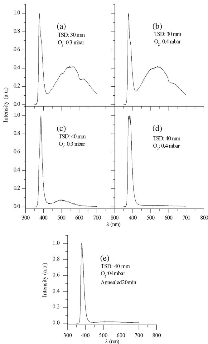
**Figure 2.** PL spectra of grown thin film with expected blue band-edge transition (about 370 nm). Some of films present yellow–green and orange bands of 450–700 nm associated to lack of oxygen. Figures (a–d) correspond to as-grown films while figure (e) corresponds to a film annealed for 20 min with same oxygen pressure and temperature as used during its growth.
