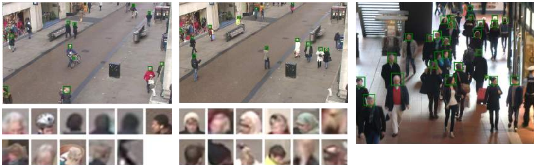
Figure 4: Some examples of detections on test images (1 + 2 town centre, 3 test image from the training set) for the final person detector.
