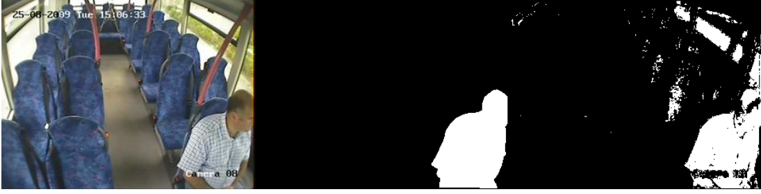
Figure 1: Typical CCTV image, the corresponding ground truth and a typical background subtraction output
