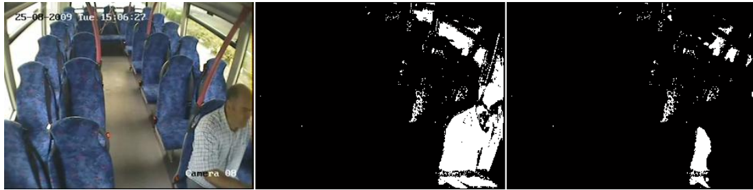
Figure 7: Segmentation output for an example frame when the angle of the foreground region matches the dominant angles of the bus window region. Left: Original Frame; Middle: Output of the Background Subtraction method; Right: Final Output combining the Optical flow and Background Subtraction outputs
