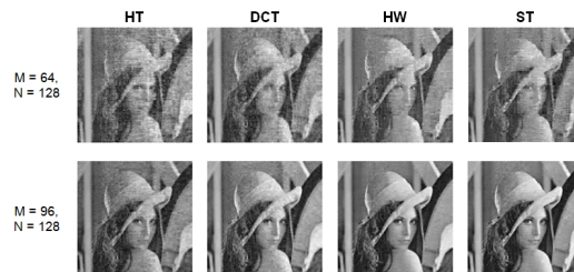
Figure 2: Payload reconstruction: \Phi of size M \times N and (HT, DCT, HW, ST) of size N \times N .
