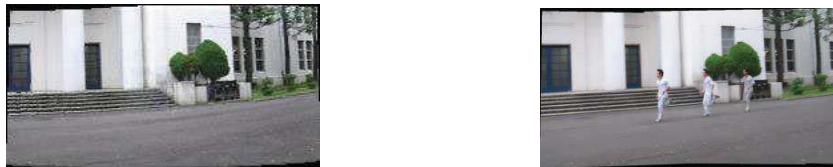
(a) Stitched image extracted only background (b) Stitched image projected runners in each frame
