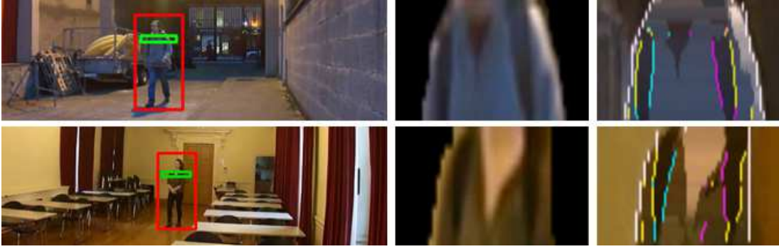
Figure 3: Successful detections of backpacks in individual frames in twilight conditions (top row) and indoor with low level of contrast relative to the underlying clothing (bottom row).
