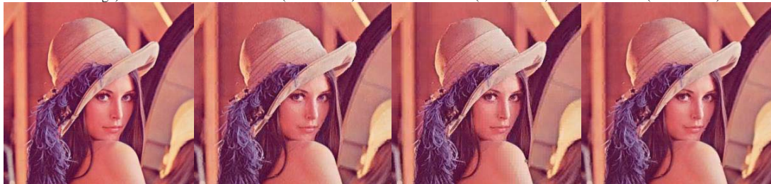
Fig. 8. (a) Original Image (Std. test Image) Fig. 8. (b) Image coded using QR 1:2:3:4:5 (CR = 31.13). Fig. 8. (c) Image coded using QR 5:4:3:2:1 (CR = 36.46). Fig. 8. (d) Image coded using QF 1 (CR = 24.56).
