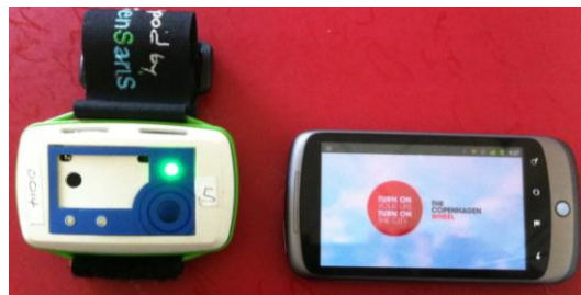
Figure 3: Ecosenspod (left) connected via Bluetooth to an android phone (right)
