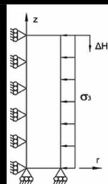
Figure 2. Triaxial compression model
