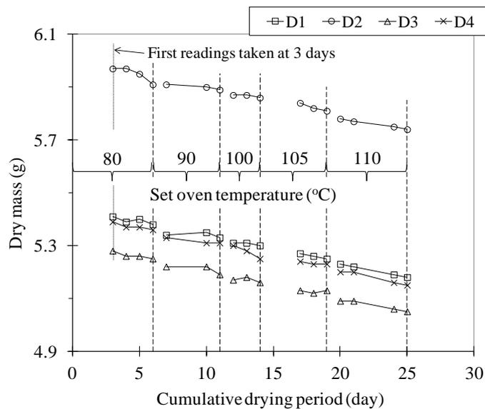
FIG. 3. Reduction in specimen dry mass against drying period for different oven temperatures.
