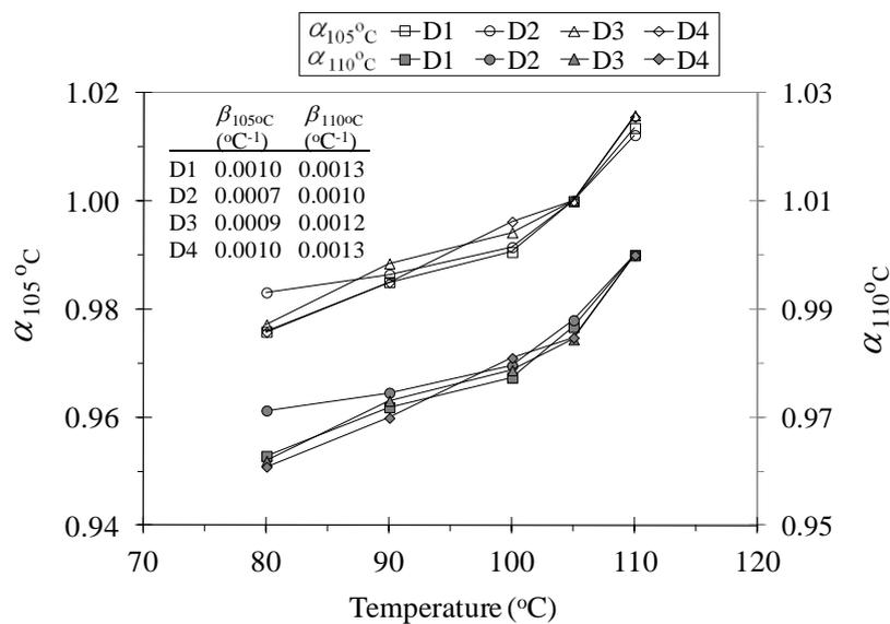
FIG. 5. Parameter  $\alpha$  against drying temperature correlations deduced from experimental data reported in literature. Note  $\alpha_{105^\circ\text{C}}$  and  $\alpha_{110^\circ\text{C}}$  correspond to reference drying temperatures of  $105^\circ\text{C}$  and  $110^\circ\text{C}$  respectively.
