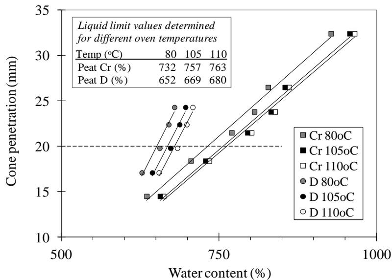
FIG. 9. Water content against undrained strength for Clara refined peat.
