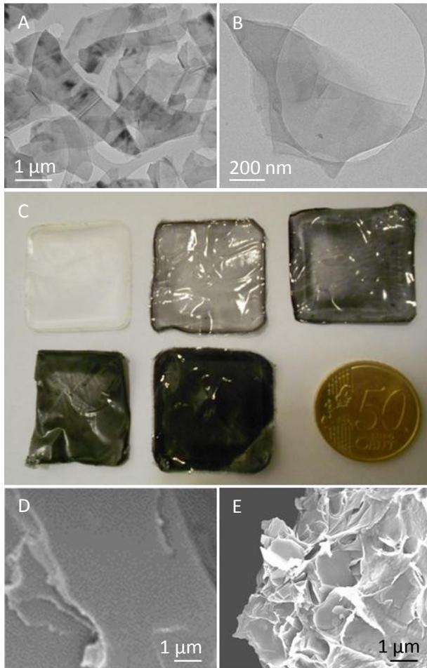
Figure 1: A) Large numbers of multilayer graphene deposited on a holey carbon TEM grid. B) An individual graphene multilayer. C) Photograph of PVAc-graphene films with mass fractions of 0%, 0.2%, 0.4%, 0.7% 1.5% (volume fractions from 0% to 0.8%). SEM image of D) a PVAc and E) a PVAc/graphene fracture surface.
