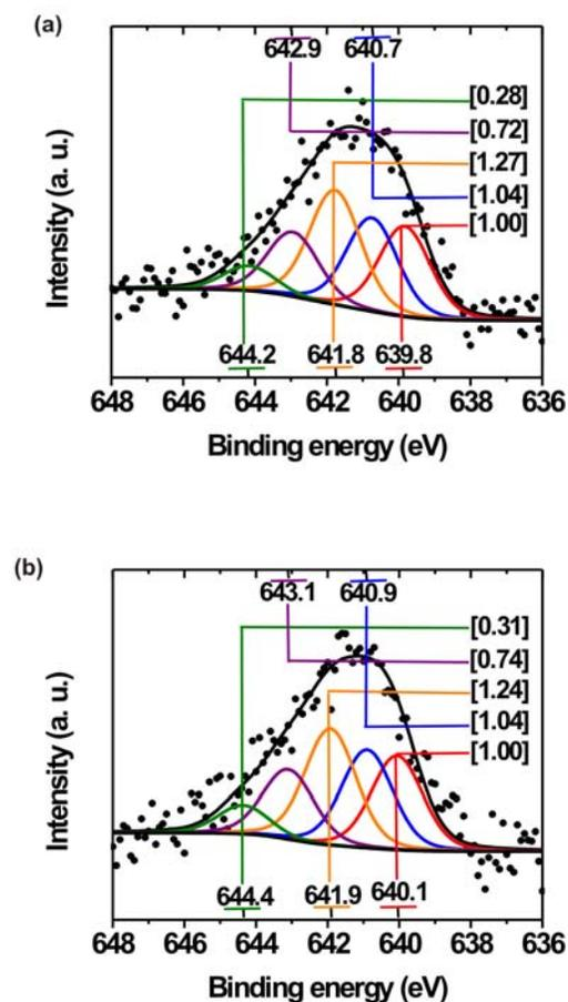
**Figure 6.** Mn  $2p_{3/2}$  XPS spectra obtained from the Cl-MnTPP monolayer on the Ag(111) surface (a) as deposited, and (b) after the complete loss of the Cl ligand. The dots represent the spectral data. The black and grey lines correspond to the best fit to the spectral data and Shirley backgrounds respectively. Peak intensities (bracketed values) are relative to that of lowest binding energy.
