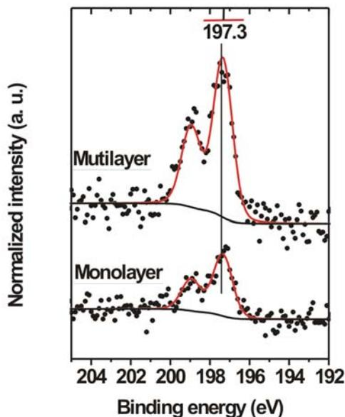
**Figure 4.** Cl 2p XPS spectra obtained from the Cl-MnTPP overlayer on the Ag(111) surface at a coverage of  $\sim 1$ ML (lower) and  $\sim 2.5$  ML (upper). The dots represent the spectral data. The red and black lines correspond to the best fit to the spectral data and Shirley backgrounds respectively.
