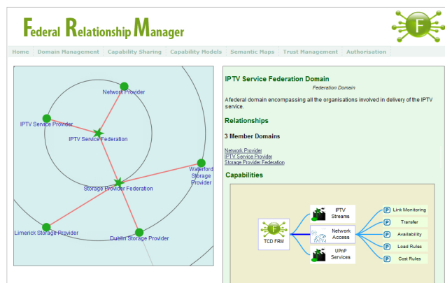
Fig. 7 A screen snapshot of the Federal Relationship Manager interface; a visualisation of federation membership is shown on the left, whilst the right shows details of capability models.
