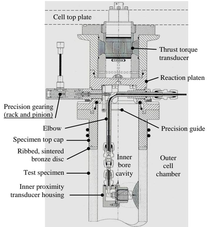
Figure 5. Mechanism that locates inner proximity transducer.
