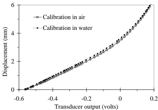
Figure 8. Comparison of calibration in water and in air.
