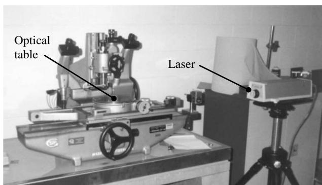
Figure 6. Optical table and laser distance measurement system.
