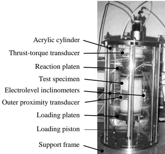
Figure 1. Cell of UCD hollow cylinder apparatus.
