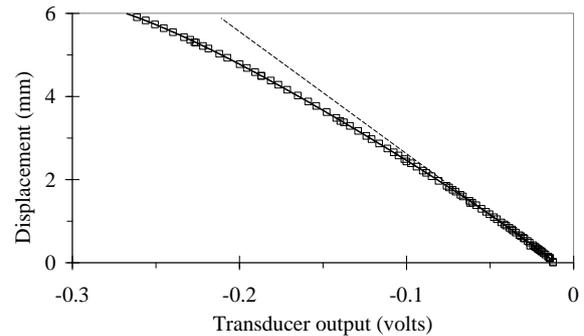
(a) Outer proximity transducer and convex target.
