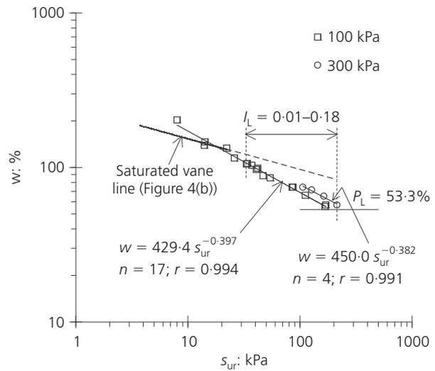
Figure 5. Water content against undrained strength in triaxial compression under cell pressures of 100 and 300 kPa
