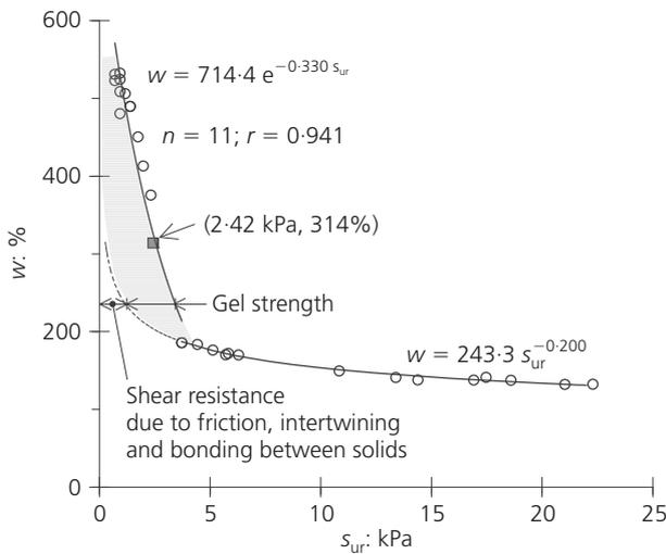
Figure 12. Water content against vane strength for material of slurry to soft consistency
