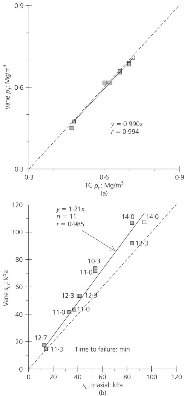
Figure 9. Effect of shearing mode on deduced strength: (a) dry density; (b) remoulded strength
