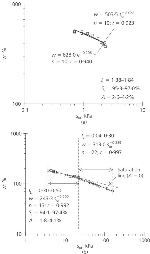
Figure 4. Water content against strength in vane shear: (a) slurry material; (b) plastic material
