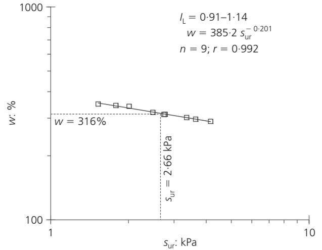
Figure 3. Water content against dynamic shear strength from fall-cone tests ( $n$ , number of data points;  $r$ , regression coefficient)
