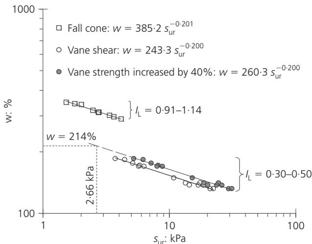
Figure 10. Water content against undrained strength adjusted for difference in strain rate
