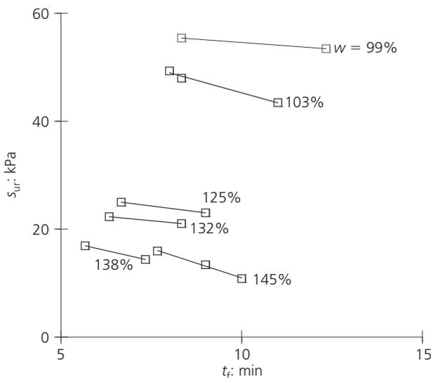
Figure 7. Vane  $s_{ur}$  mobilised for different times to failure
