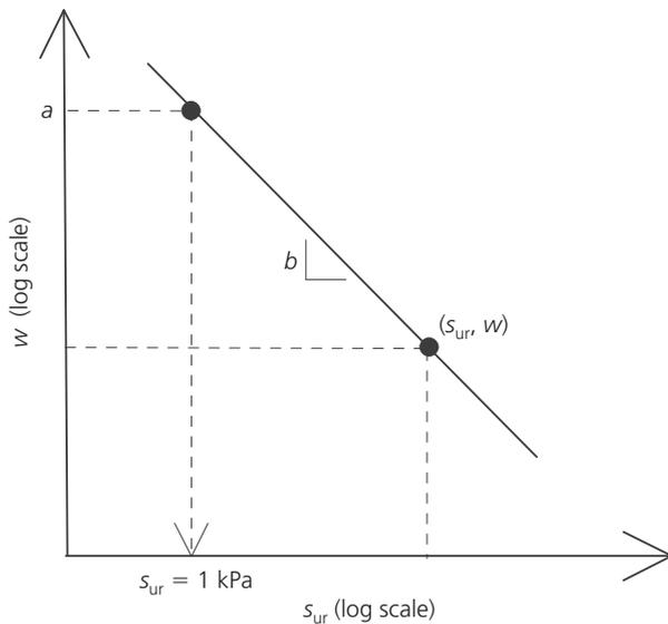
**Figure 1.** Water content against remoulded undrained shear strength for fine-grained mineral soil
