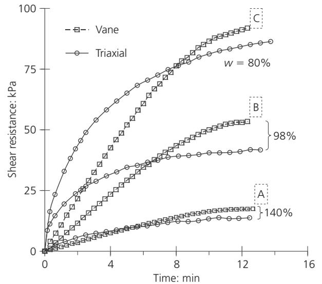
Figure 8. Response of identical specimen pairs in vane shear and TC (TC specimens deemed to have failed after a period of 12.5 min, corresponding to 20% axial strain)
