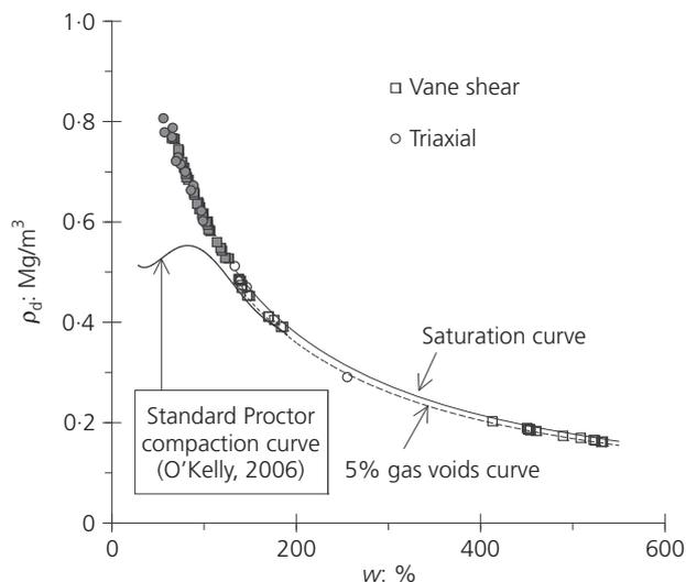
**Figure 2.** Dry density against water content for sewage sludge, including data of O'Kelly (2004b, 2006) (hollow symbols, material of slurry and soft consistencies; solid symbols, compacted air-dried material)
