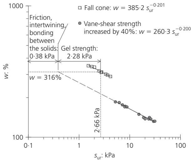
Figure 11. Fall-cone and vane data adjusted for difference in strain rate
