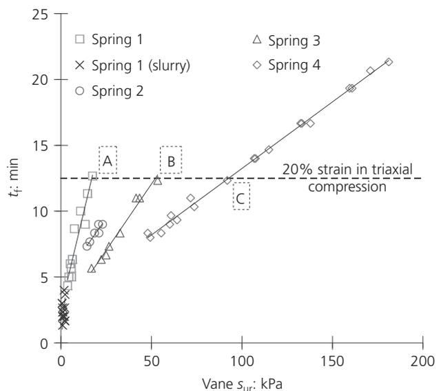
Figure 6. Time to failure in vane shear for different water contents and torsion springs (stiffness of springs in order 1 to 4 was 1.0, 1.9, 3.3 and 5.8 kN/m<sup>2</sup>)
